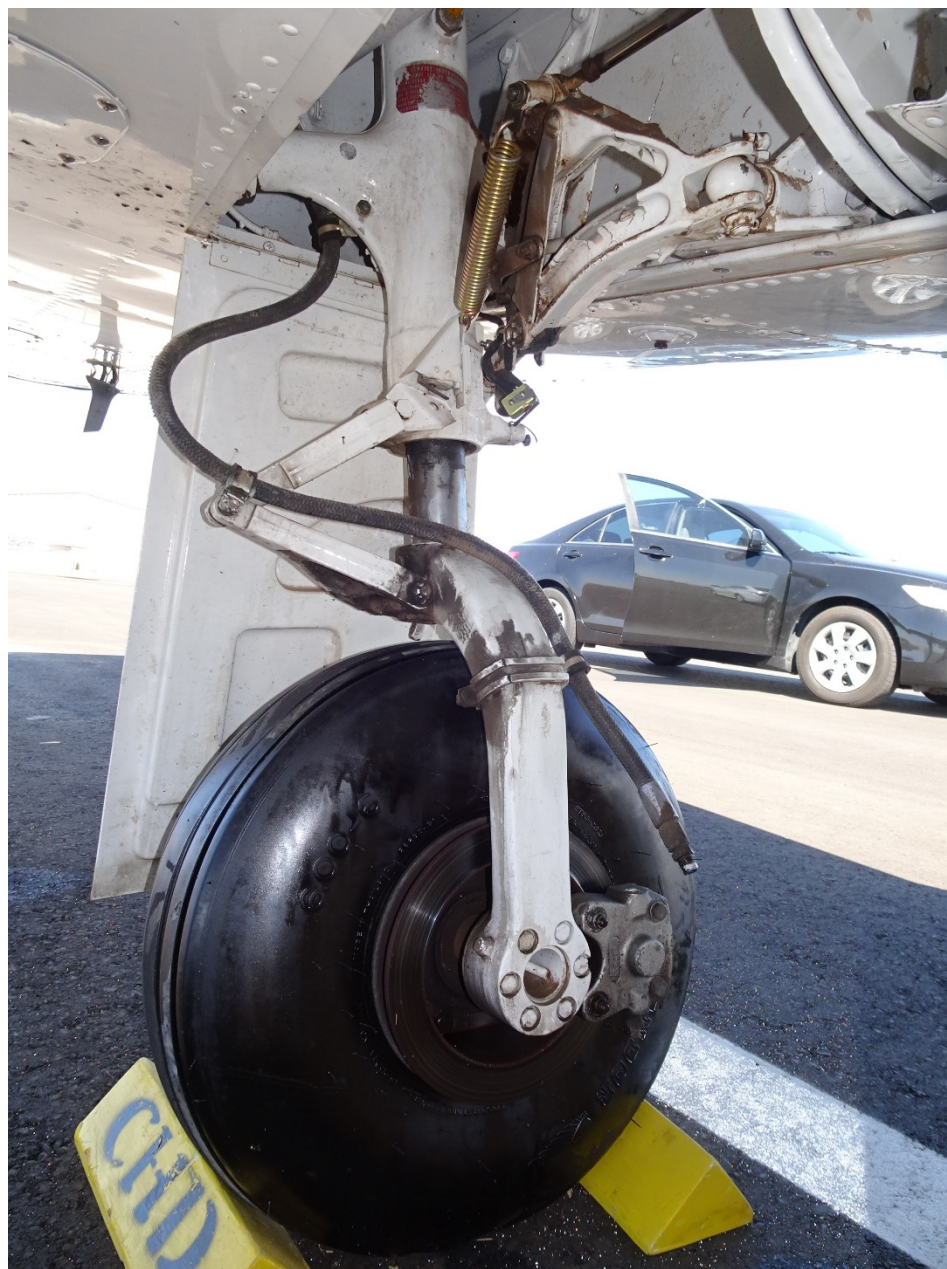
Photo 2 - View of extended left main landing gear with a bent upper side brace link
