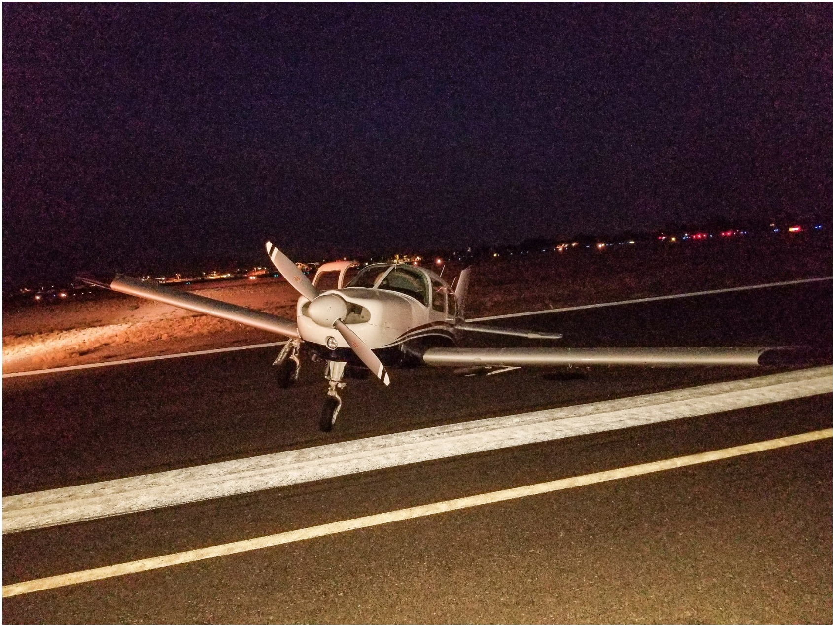
Photo 1 – View of airplane on the runway with a collapsed left main landing gear
