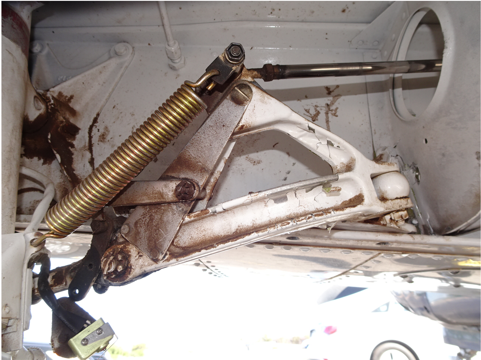
Photo 3 – Closeup view of bent left main landing gear upper side brace link
