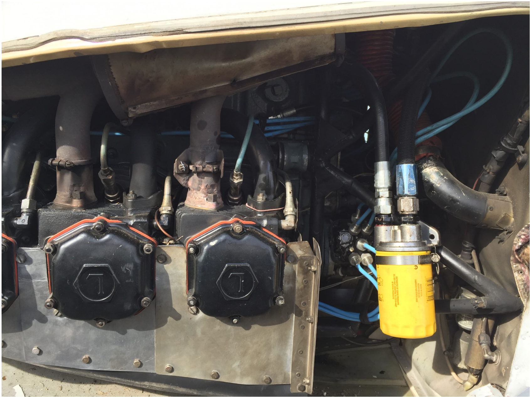
Photo 4 – View of right side of inverted engine with automotive oil bypass filter (courtesy of the FAA)
