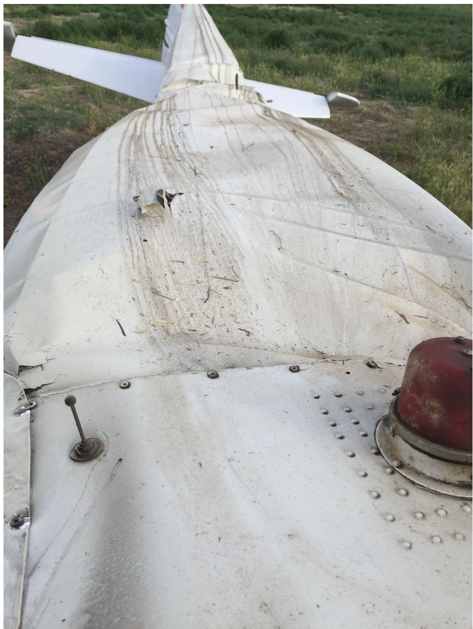
Photo 2 – View of oil residue on the belly of the airplane (courtesy of the FAA)
