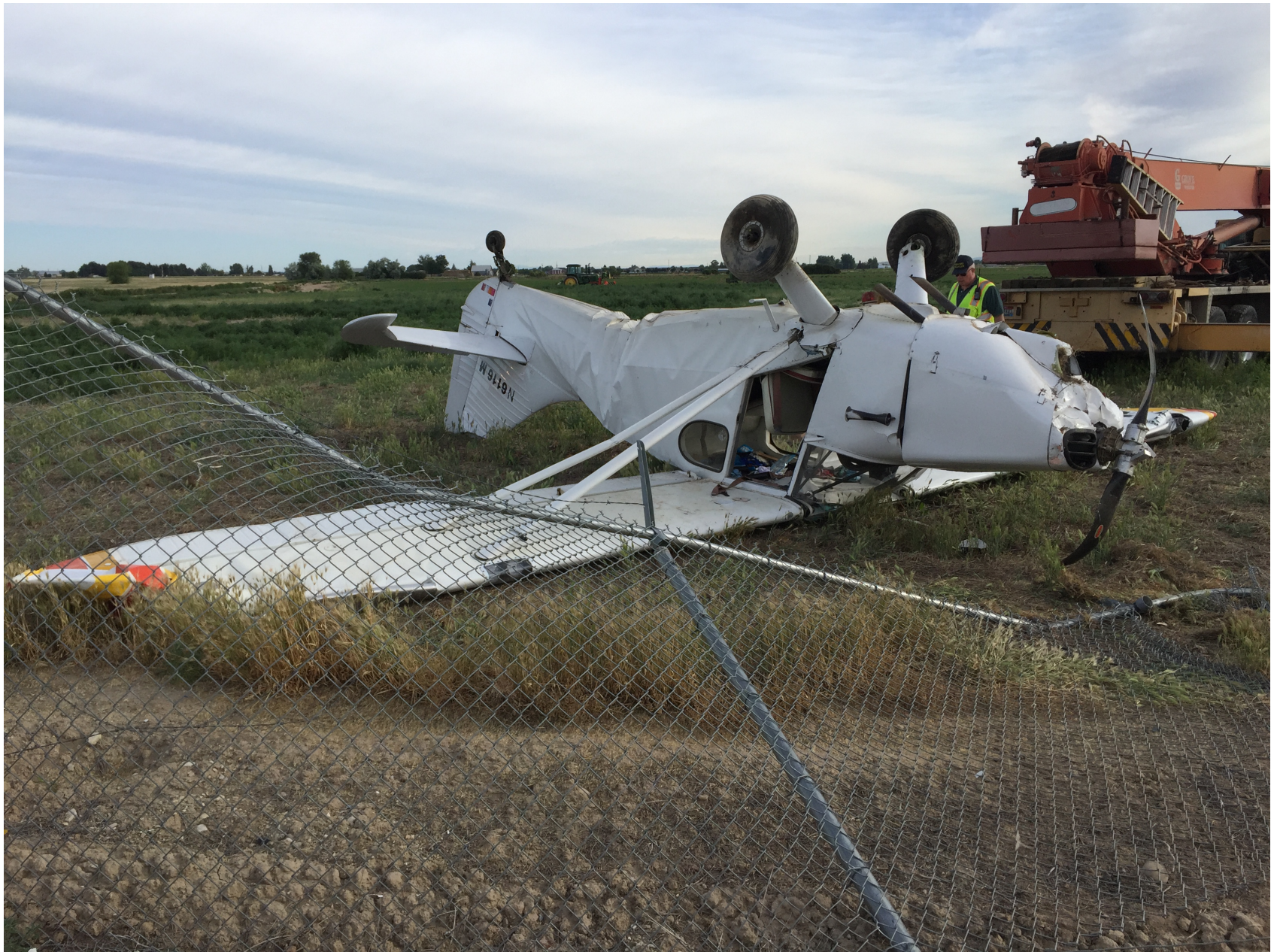
Photo 1 – View of inverted airplane with damaged fuselage (courtesy of the FAA)
