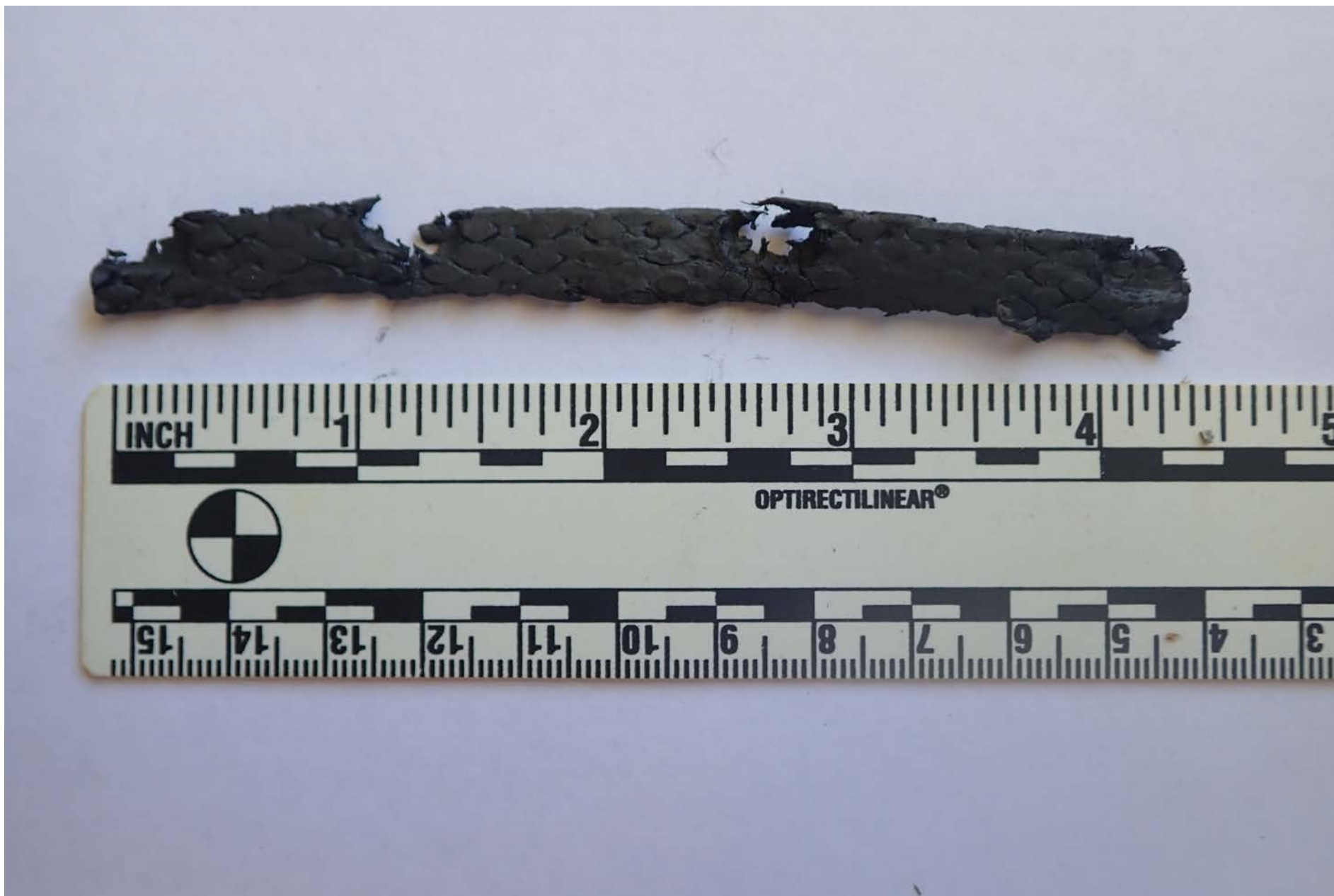
Photo 5 –Valve Seal Material
