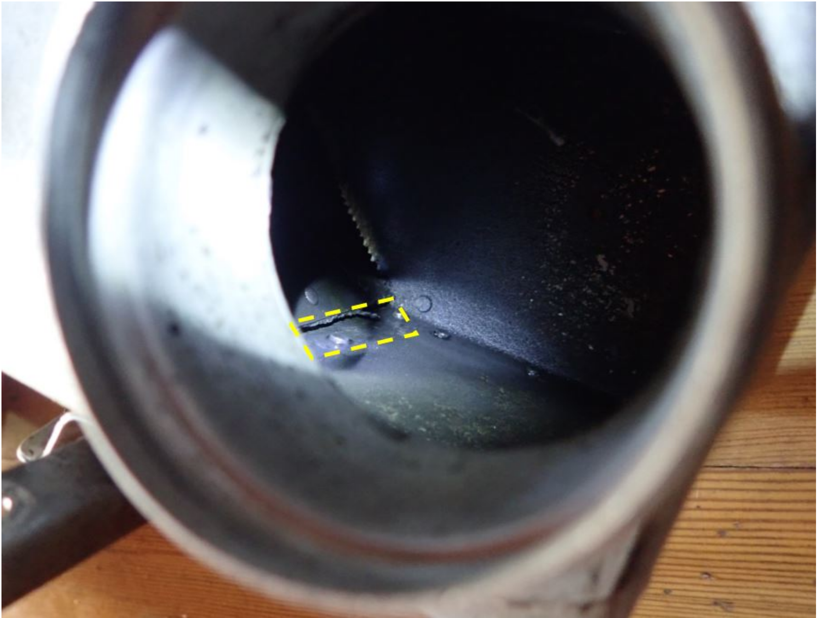
Photo 8 - Carburetor Heat Butterfly Valve with Carb in the Heat ON Position. Viewed from Hot Air Inlet. Missing Seal Highlighted.
