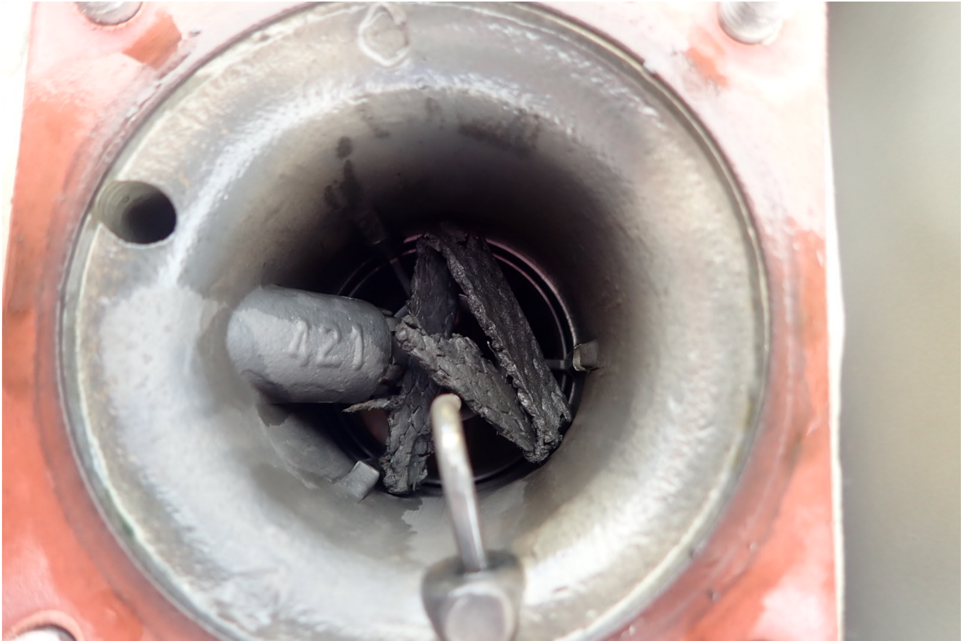
Photo 4 – Carburetor Venturi with Valve Seal
