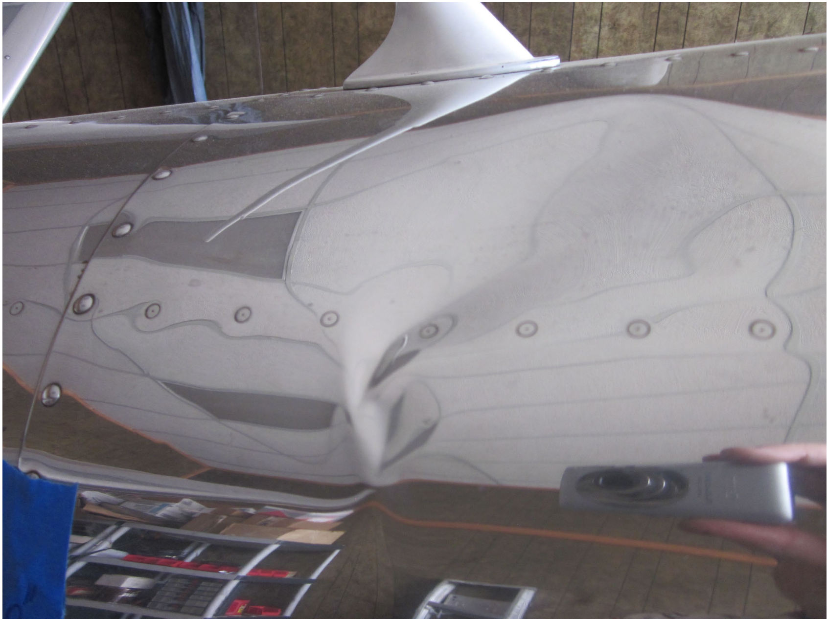
Photo 1 – Fuselage Damage Right Side (FAA Photo)
