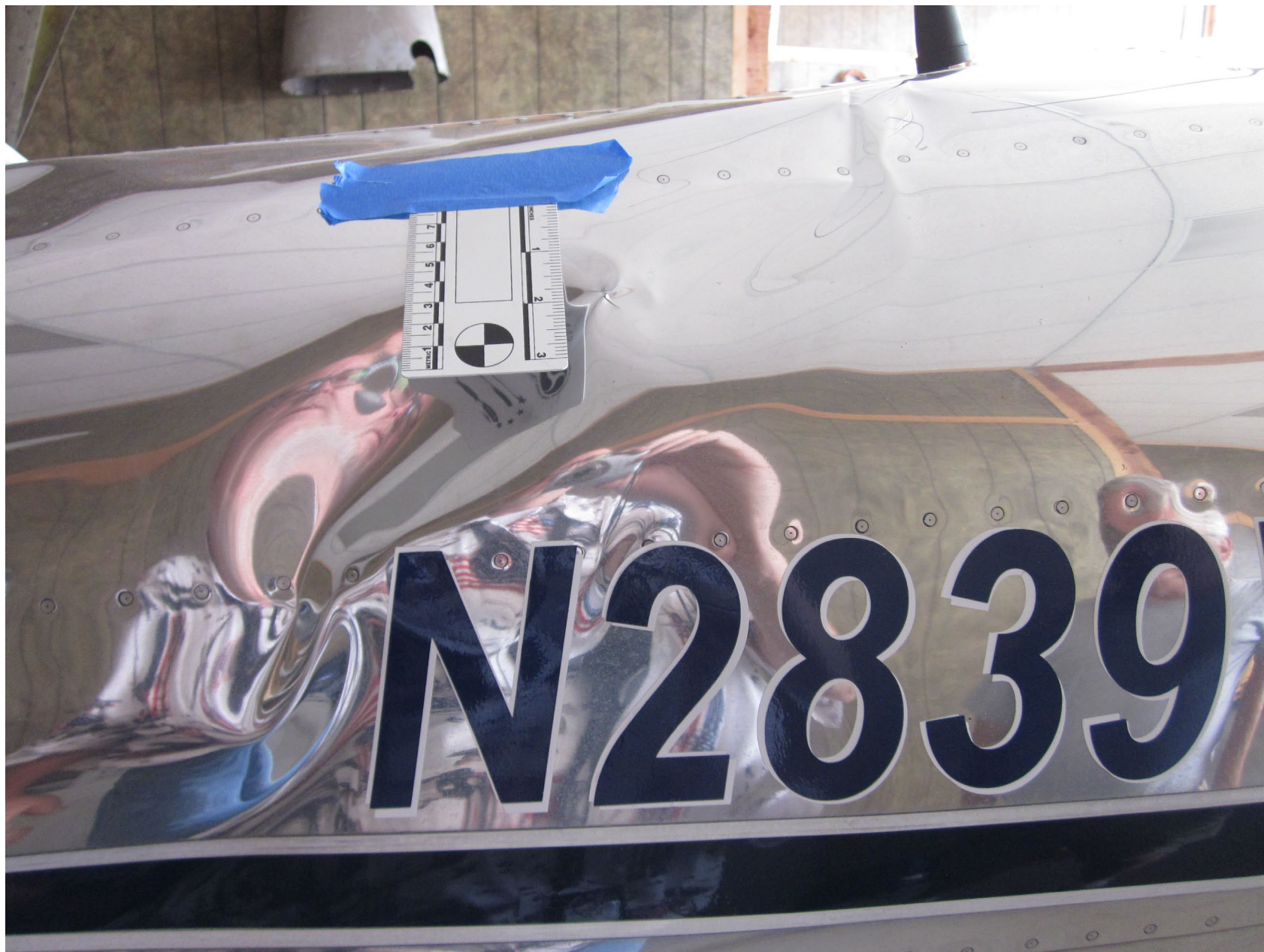
Photo 2 – Fuselage Damage Forward Right Side (FAA Photo)
