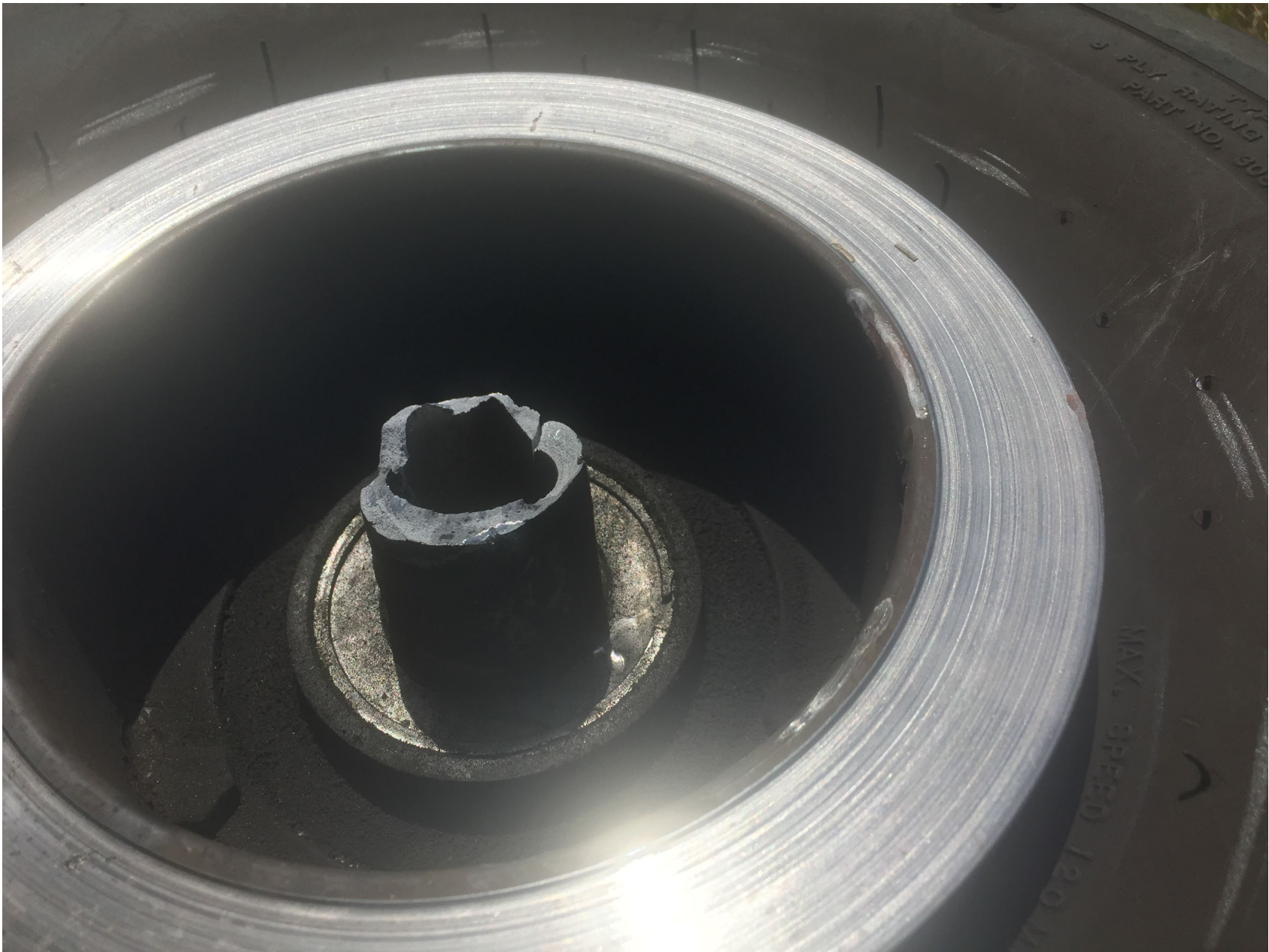
Photo 2 – Separated Landing Gear Axle at the Wheel (Photo Courtesy of FAA)
