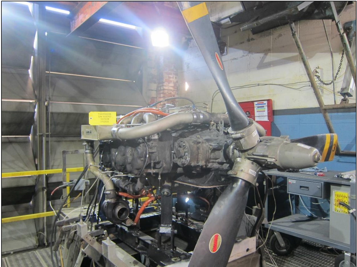
Figure 8-Engine installed on a test stand.
