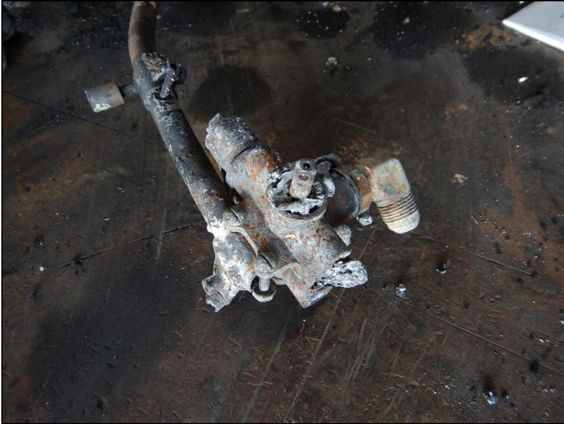
Figure 5-Followup Examination-Fuel Selector Valve
