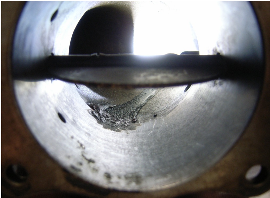
Figure 4 - Throttle Bore Deposits (Downstream of cleaned area)
