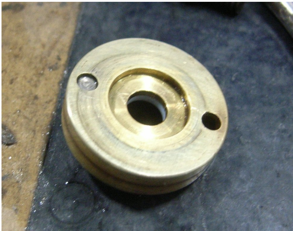
Figure 2 - Metering Plug (mating surface, prior to lapping)
