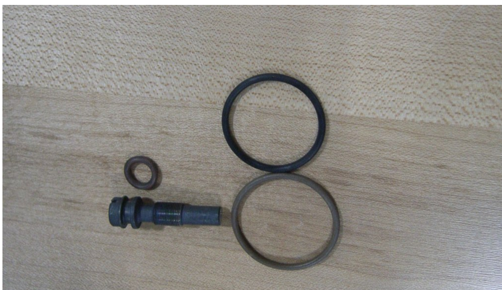
Figure 3 – Removed Idle Mixture Screw (cleaned) and MA O-Rings
