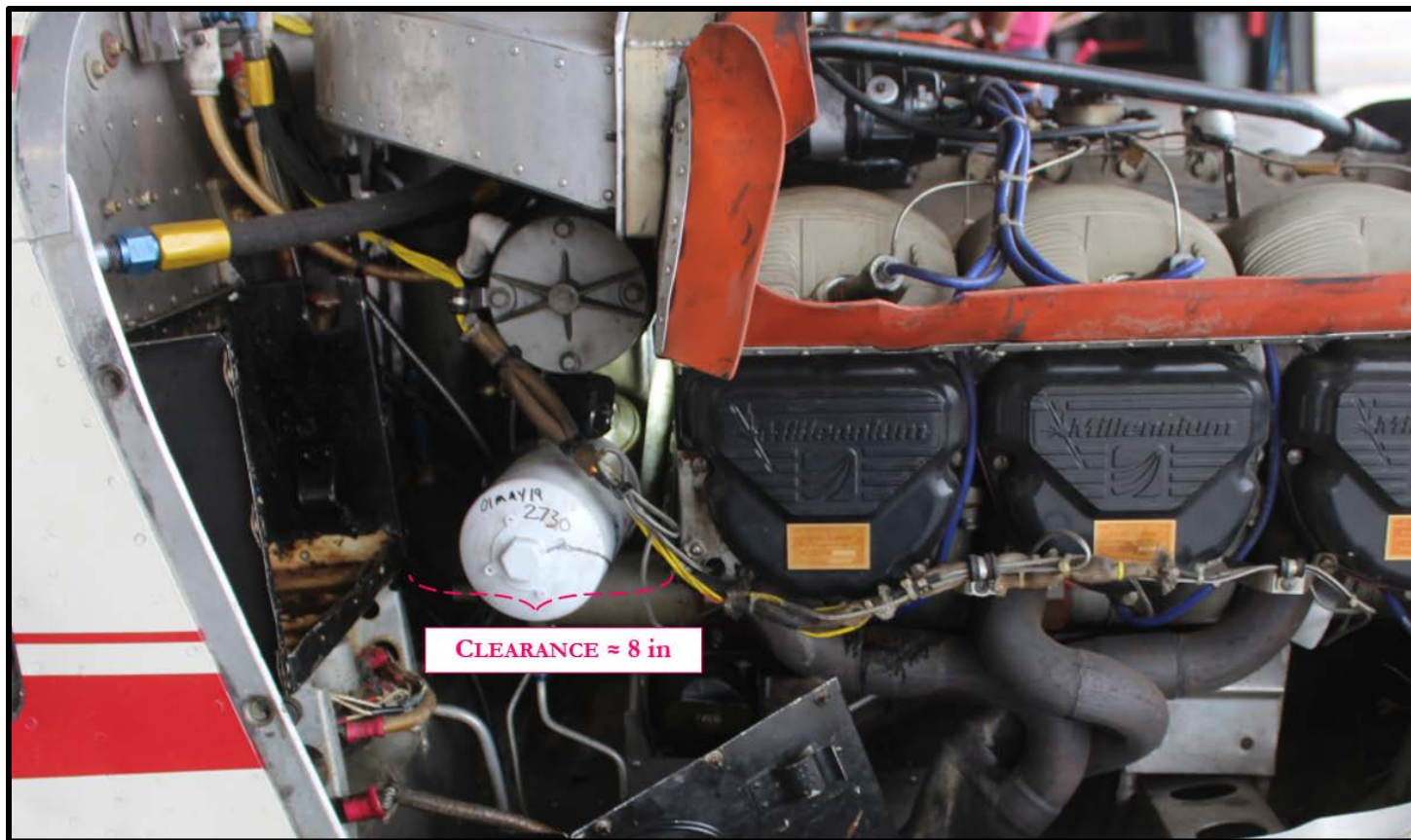
Figure 18: Clearance to Install Adapter with All Components Installed
