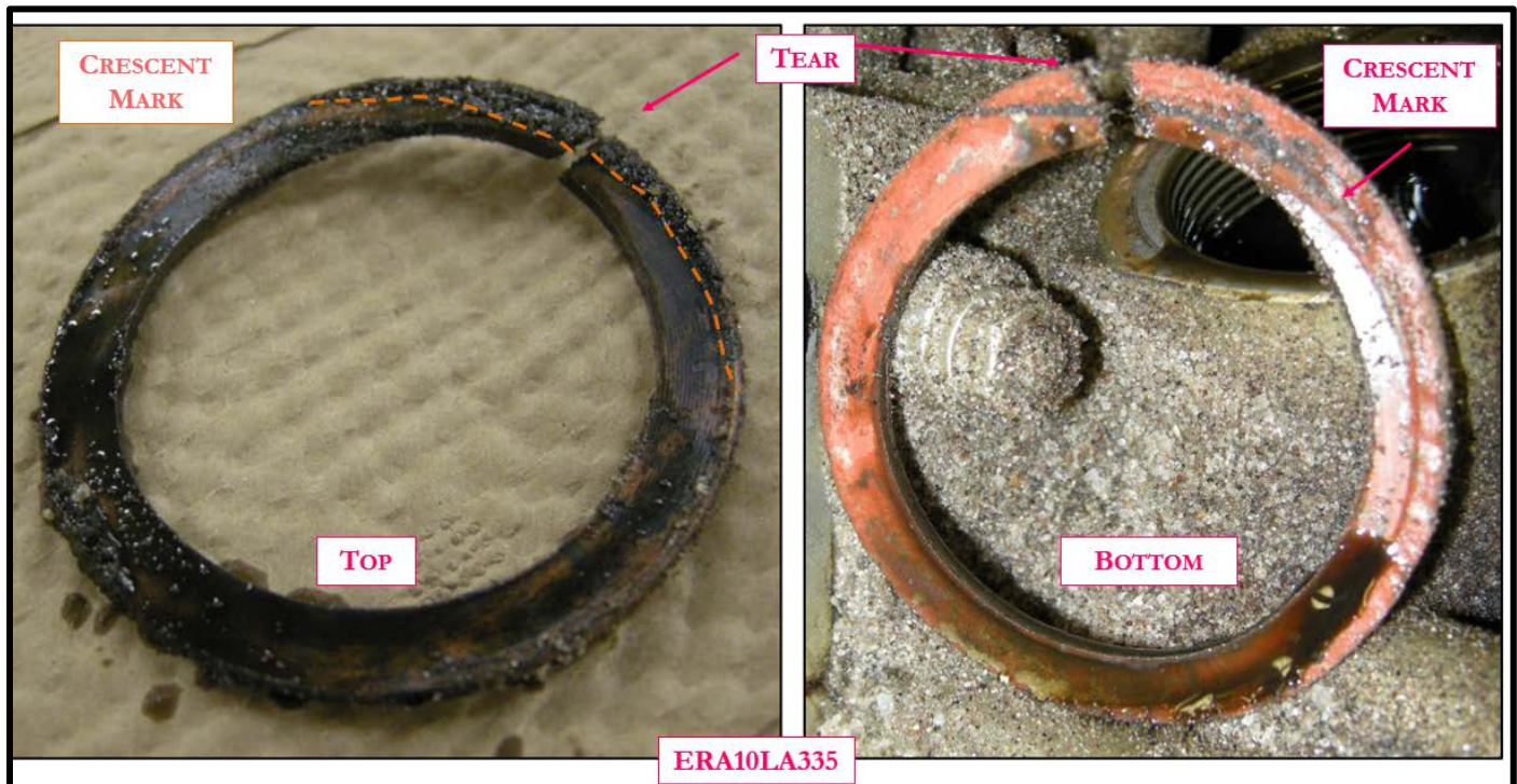
Figure 32: Prior Accident Gasket Showing Impressions/Marks ERA10LA335
