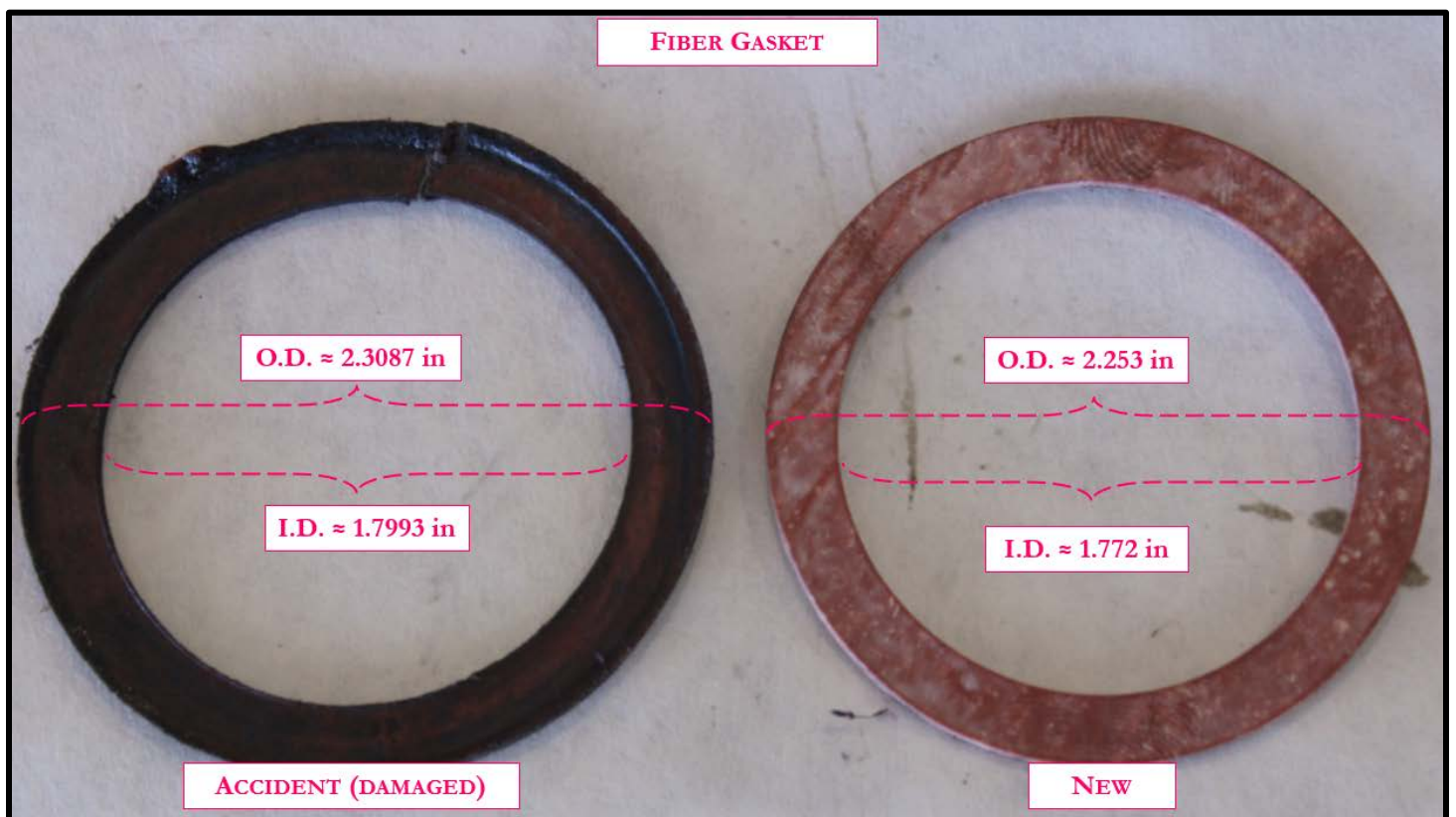
Figure 20: Fiber Gasket Measurement Comparison
