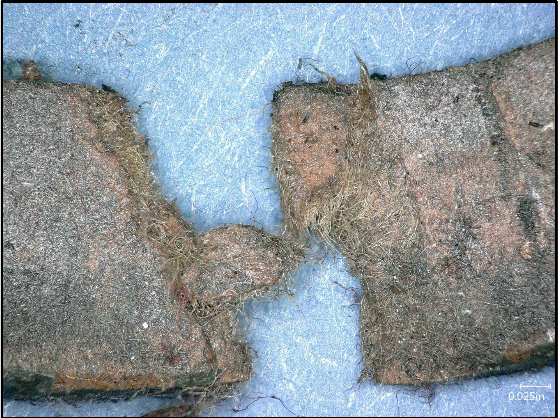
Figure 6: Fiber Gasket (tear)
