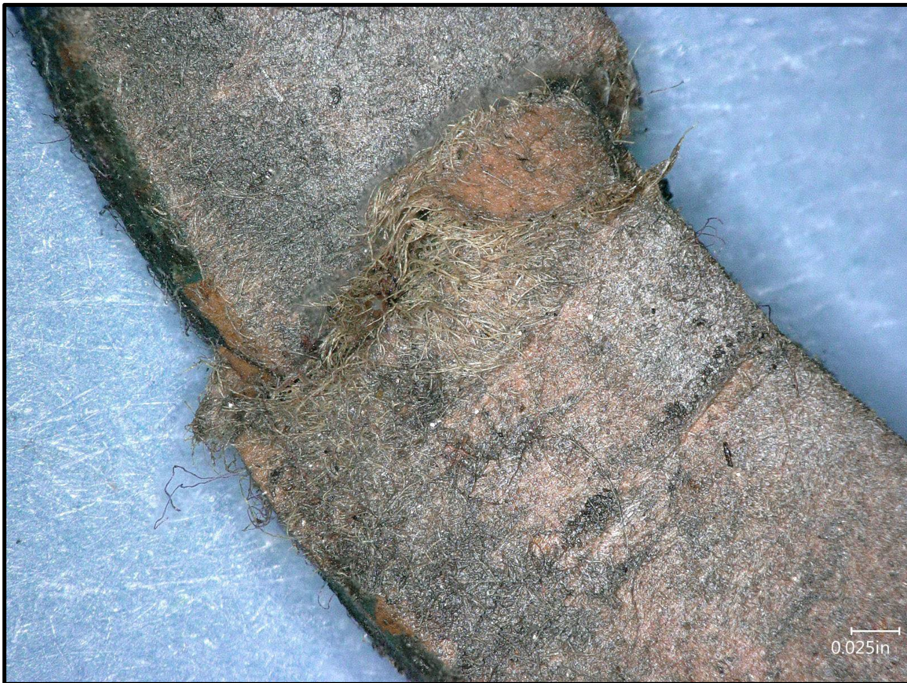
Figure 5: Tear in Gasket
