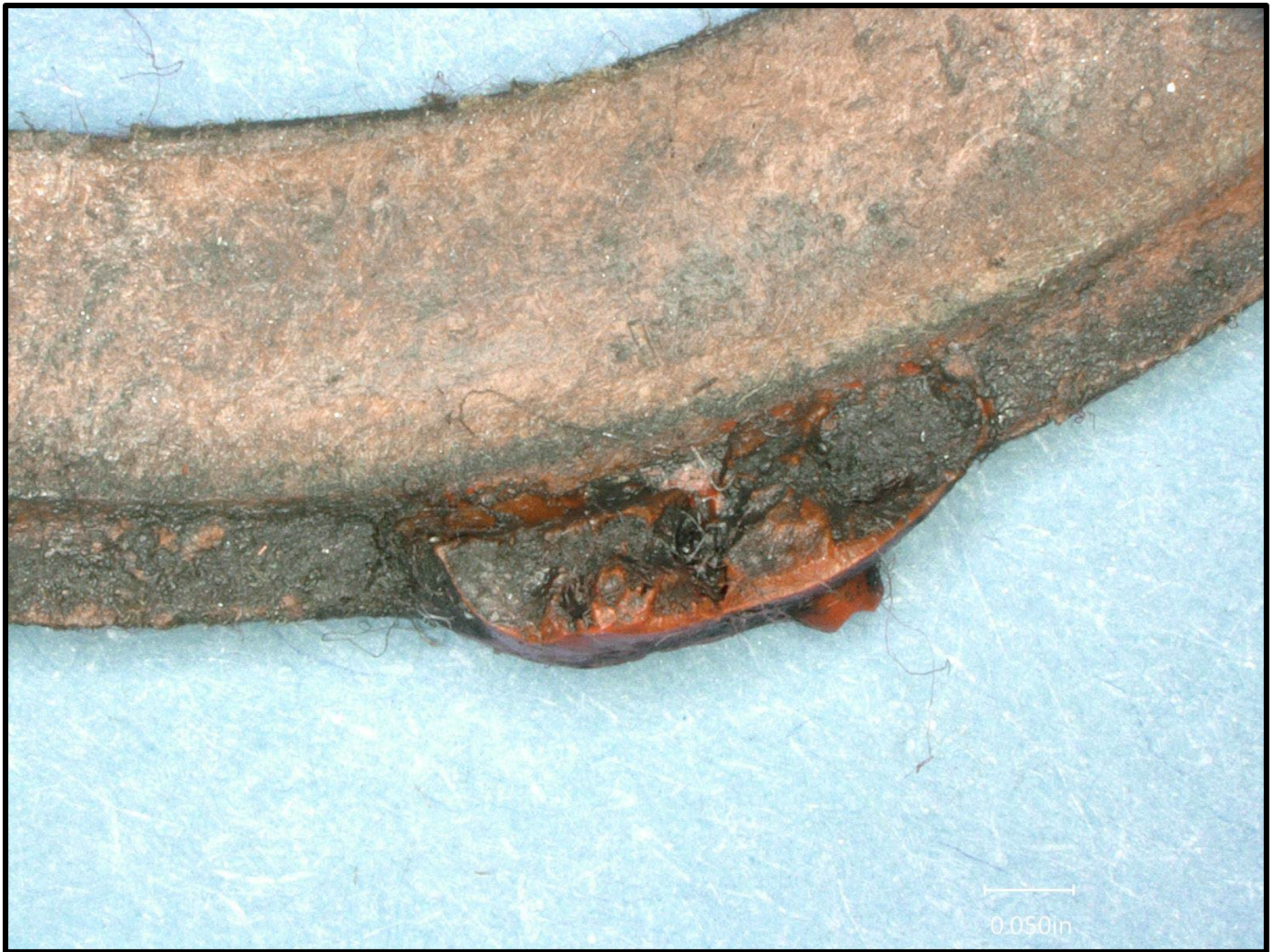
Figure 7: Fiber Gasket (showing (extrusion))
