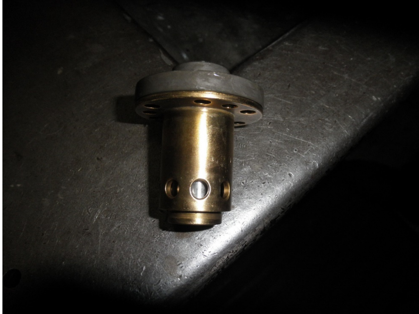
Photo No. 13: Main fuel diaphragm showing that it was intact.
