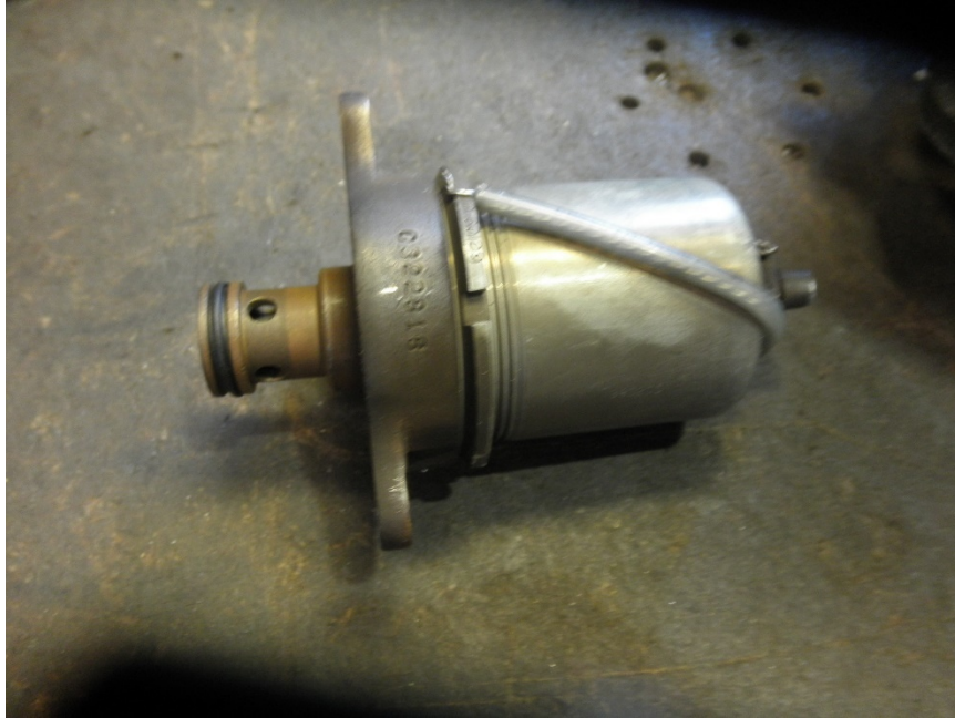
Photo No. 9: Automixture control showing O-ring that was dry was in place.
