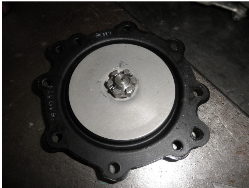
Photo No. 12: The enrichment valve showing that it was intact.
