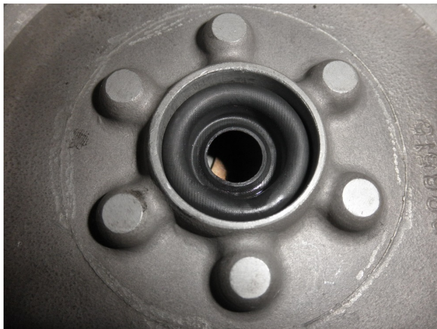
Photo No. 15: Center balance diaphragm showing that it was intact.
