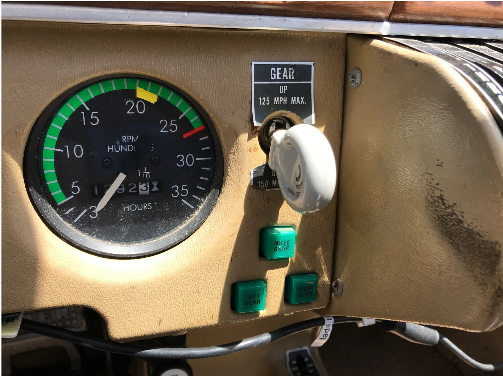
Photo 3 – Landing Gear Switch at Accident Site (Courtesy of Federal Aviation Administration)
