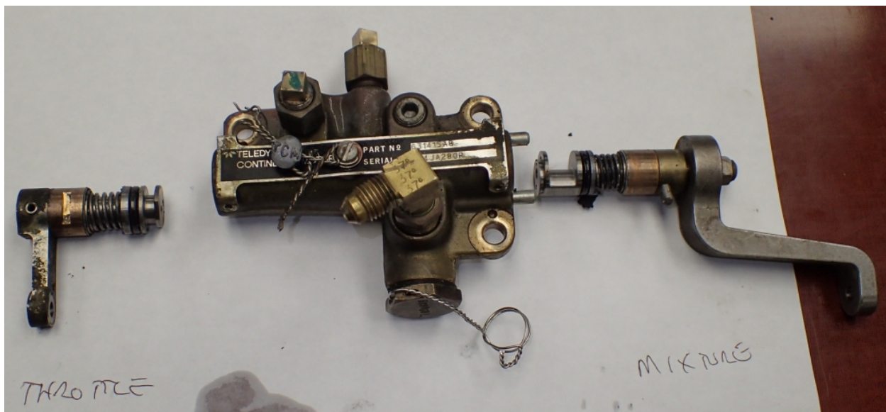
Figure 10 - Disassembled Metering Unit
