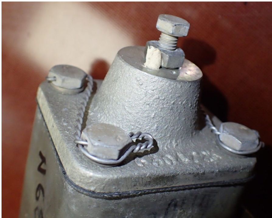
Figure 3 - EDP Adjustment Bolt (undisturbed)
