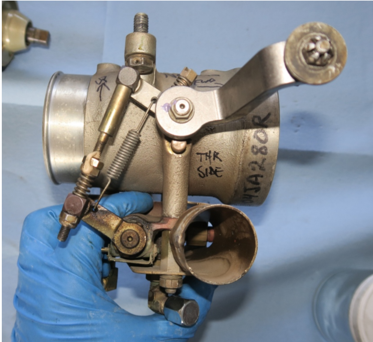
Figure 2 - T/M with Shaft Exit Staining/Grime (throttle side)
