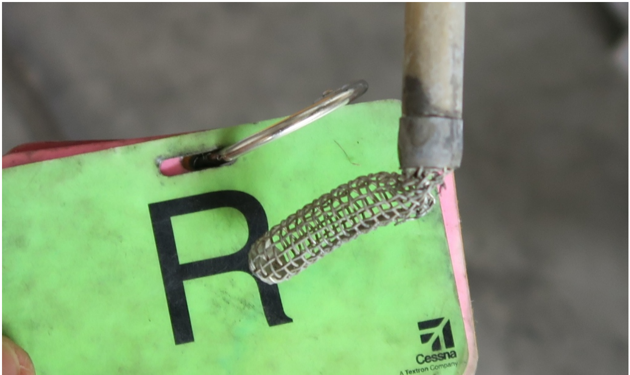
Figure 7 - Right Tank Fuel Pickup Finger Screen
