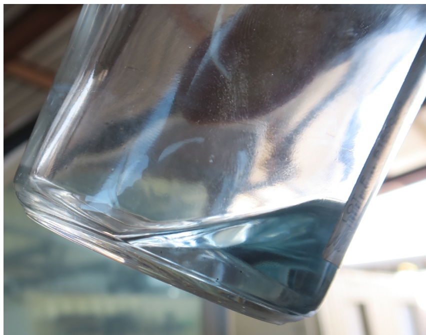
Figure 11 - Fuel Sample from Fuel Strainer
