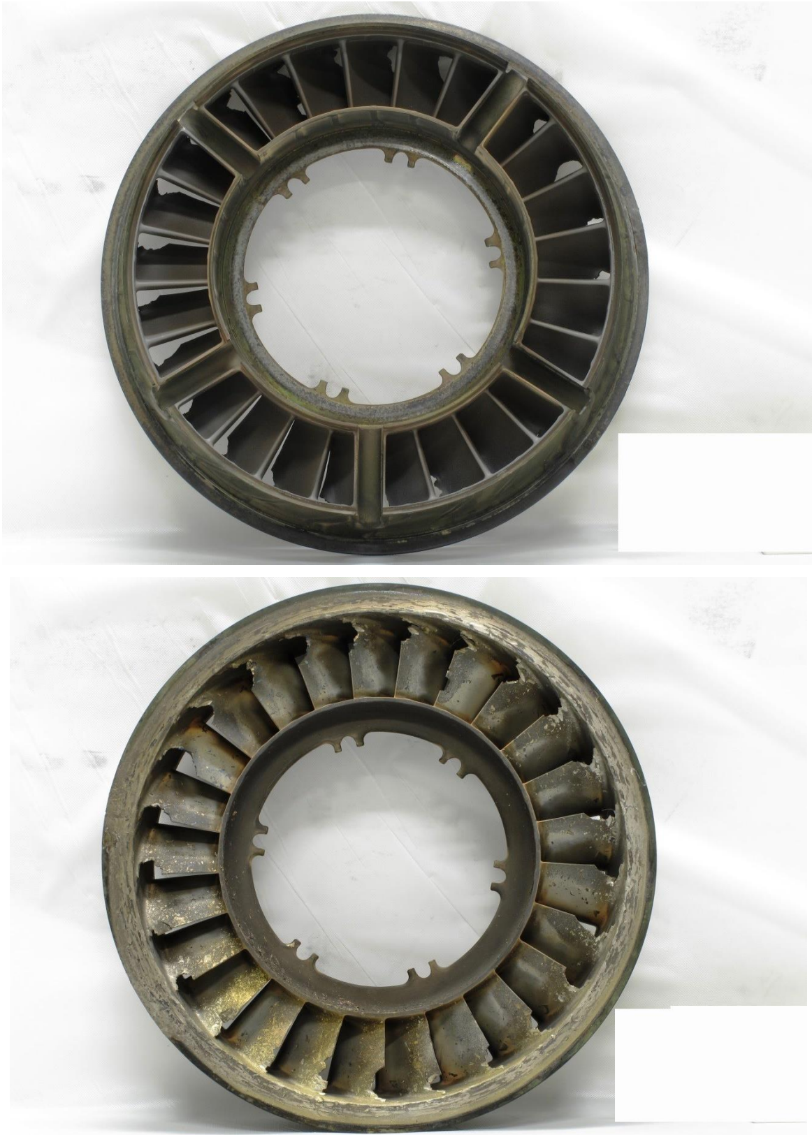
Figure 45. Leading (top) and trailing (bottom) edge side views of the third stage turbine nozzle. The suction side surfaces and trailing edges of the vane airfoils exhibited impact damage.
