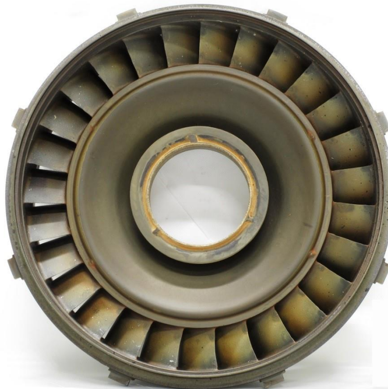
Figure 44. Leading edge (top) and trailing edge (bottom) side views of the first stage turbine nozzle. The vane airfoil suction side surfaces exhibited impact damage.
