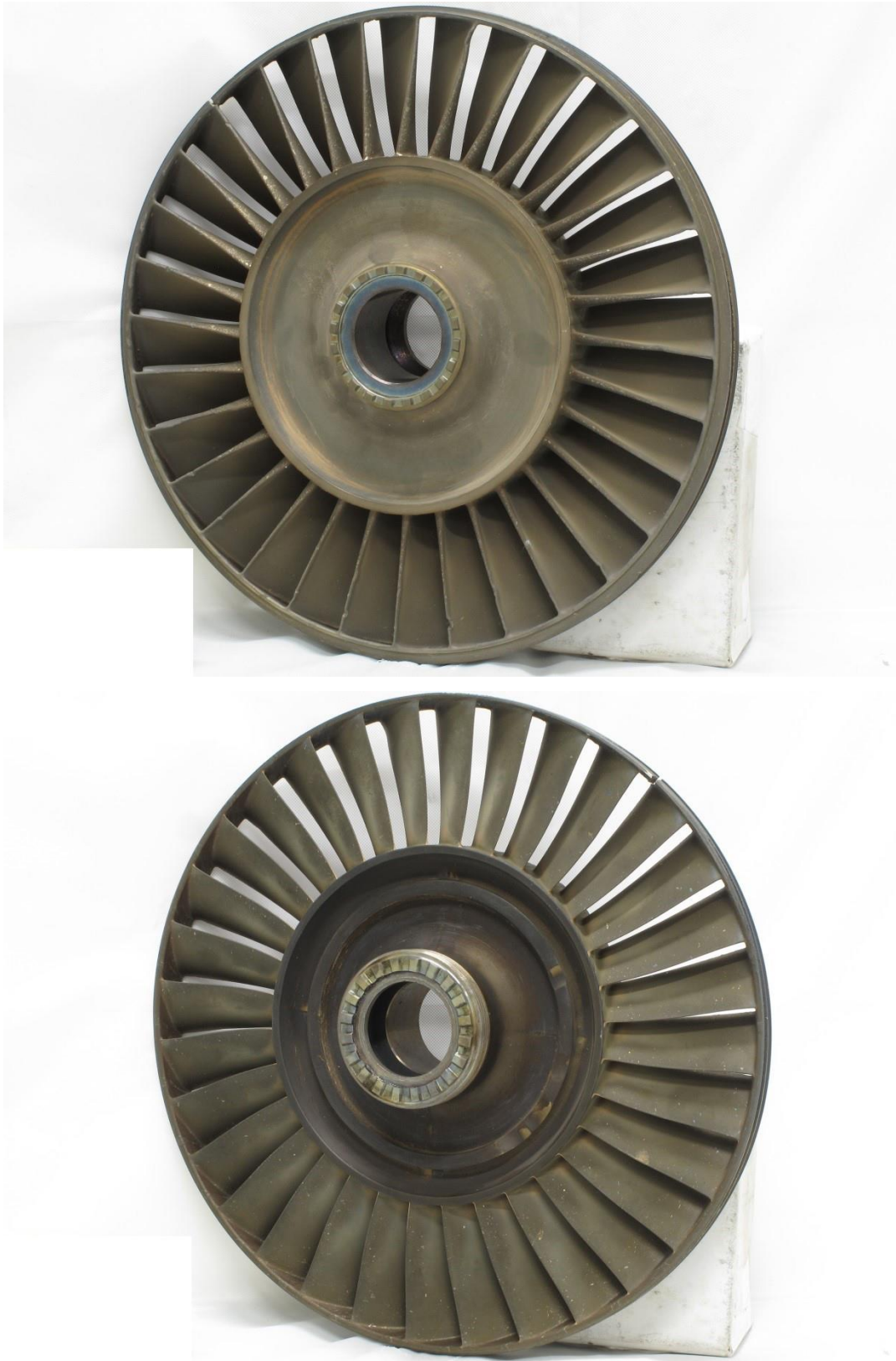
Figure 37. Leading (top) and trailing (bottom) edge side views showing the as-received condition of the fourth stage turbine wheel.
