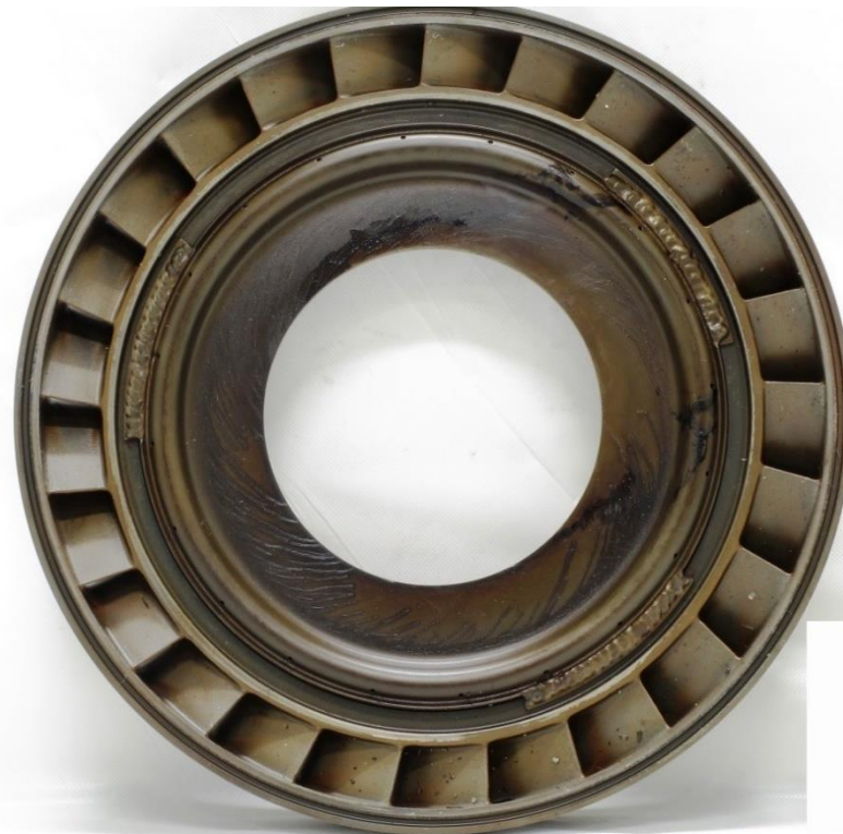
Figure 43. Leading edge (top) and trailing edge (bottom) side views of the first stage turbine nozzle. The trailing edge side web exhibited oil deposits and there was debris on the airfoils.
