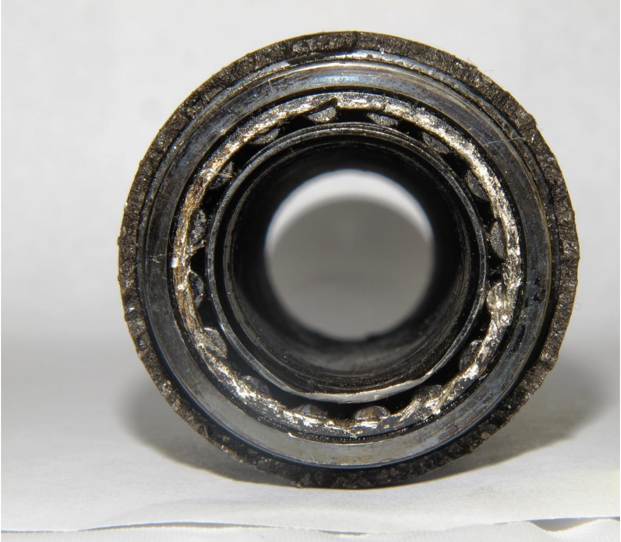
Figure 53. Aft looking forward view showing the No. 6 bearing stuck on the inner race, which is integral to the power turbine inner shaft.
