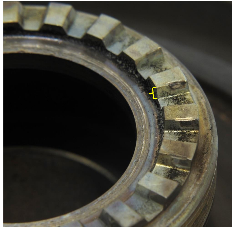
Figure 39. Detailed views showing the representative condition of the drive (left, red brace) and coast (right, yellow brace) side flanks of the turbine wheel to stub shaft curvic teeth of the fourth stage turbine wheel. The teeth exhibited patches of wear on both flanks. Coked oil was present on the curvic teeth and adjacent surfaces.
