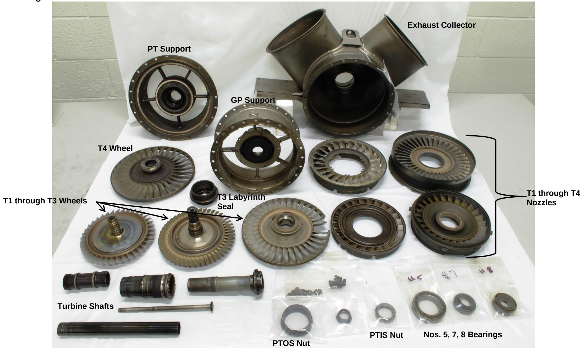
Figure 1. As-received condition of the components returned to the laboratory.
