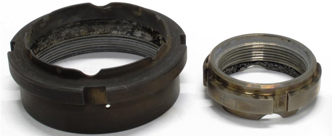
Figure 54. Power turbine outer (left) and inner (right) shaft nuts.
