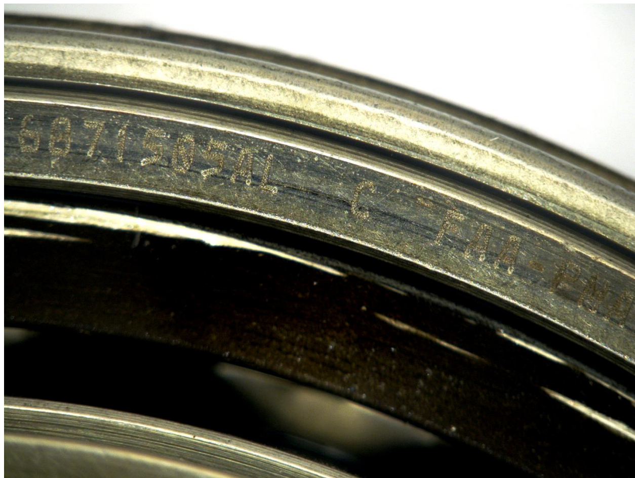
Figure 63. PMA marking (red dashed outlined area) on the No. 5 bearing.
