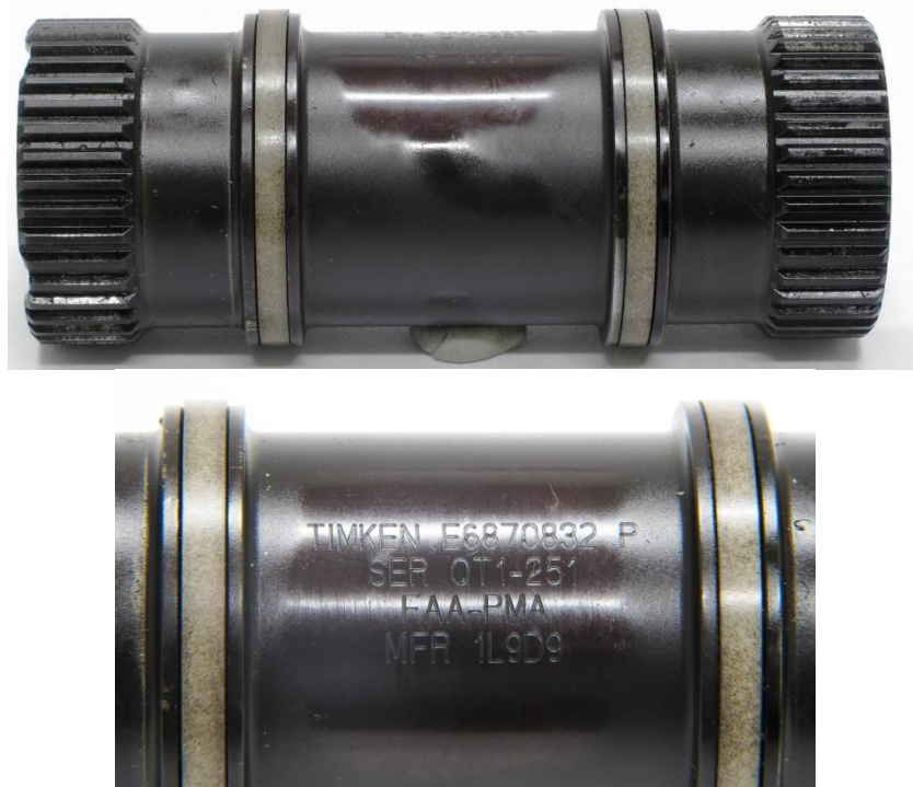
Figure 57. Photographs of the turbine to pinion gear coupling, which was a PMA component and not examined in detail.
