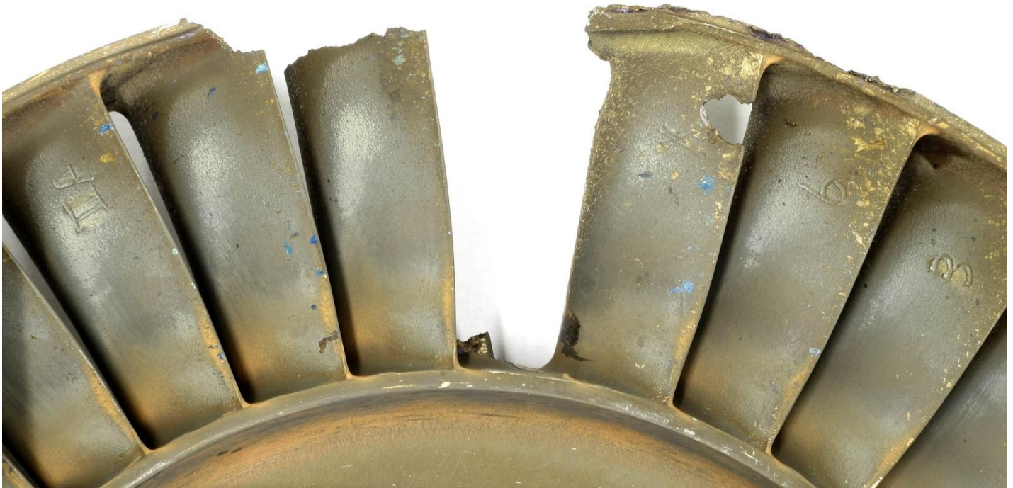
Figure 5. Detailed trailing edge view showing the fractured airfoils and shroud adjacent to the liberated airfoil on the third stage turbine wheel.
