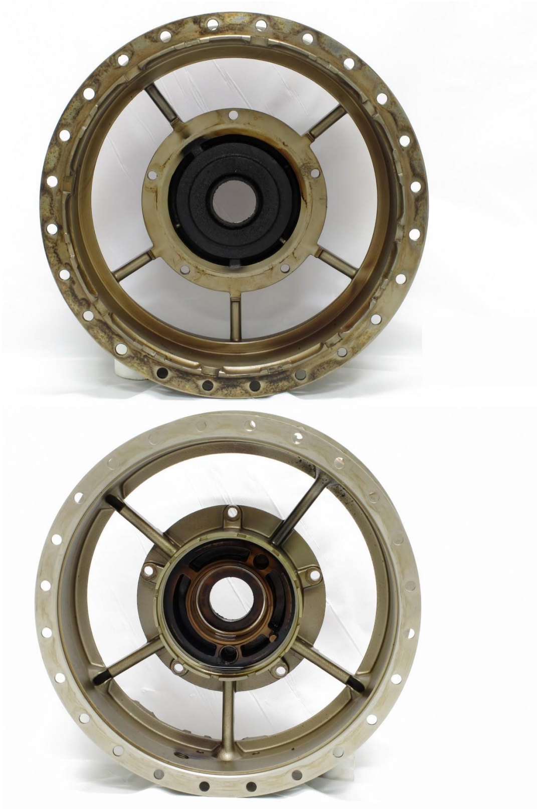
Figure 50. Forward (top) and aft (bottom) side views showing the gas producer turbine support.
