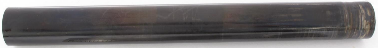
Figure 58. As-received condition of the turbine to compressor coupling. Orientation was not maintained.
