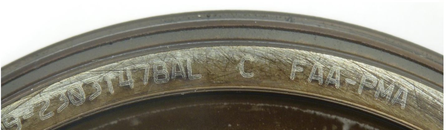
Figure 61. Forward looking aft view (top) showing the as-received condition of the No. 8 bearing, which was a PMA component (bottom).
