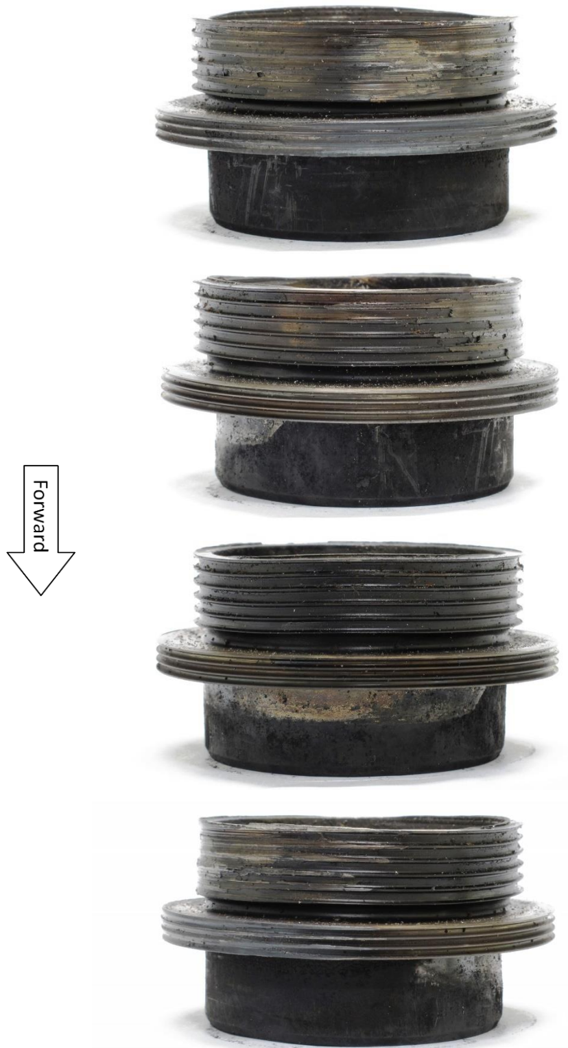
Figure 55. 90° rotated views of the third stage power turbine labyrinth seal. The seal exhibited asymmetric rub, with the most severe rub damage shown at top.
