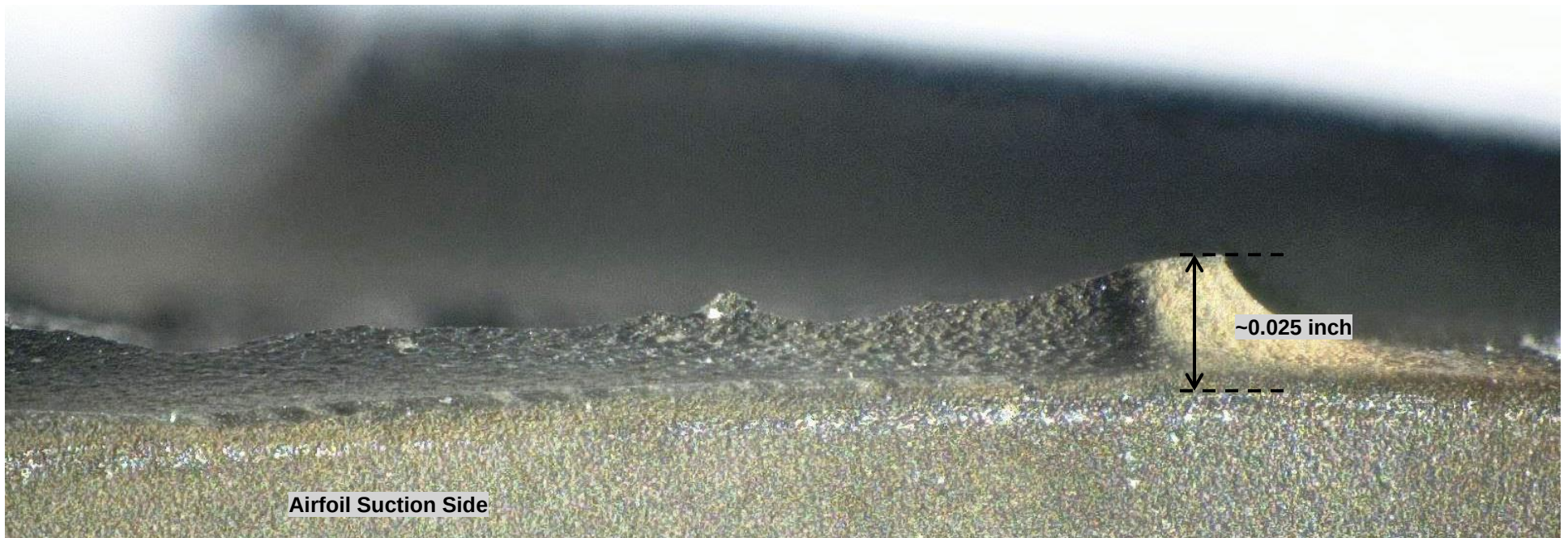
Figure 19. Detailed trailing edge view of airfoil #1 showing the geometry of the fillet and the profile of the fracture surface. The fracture initiated approximately 0.025 inch outboard of the rim.
