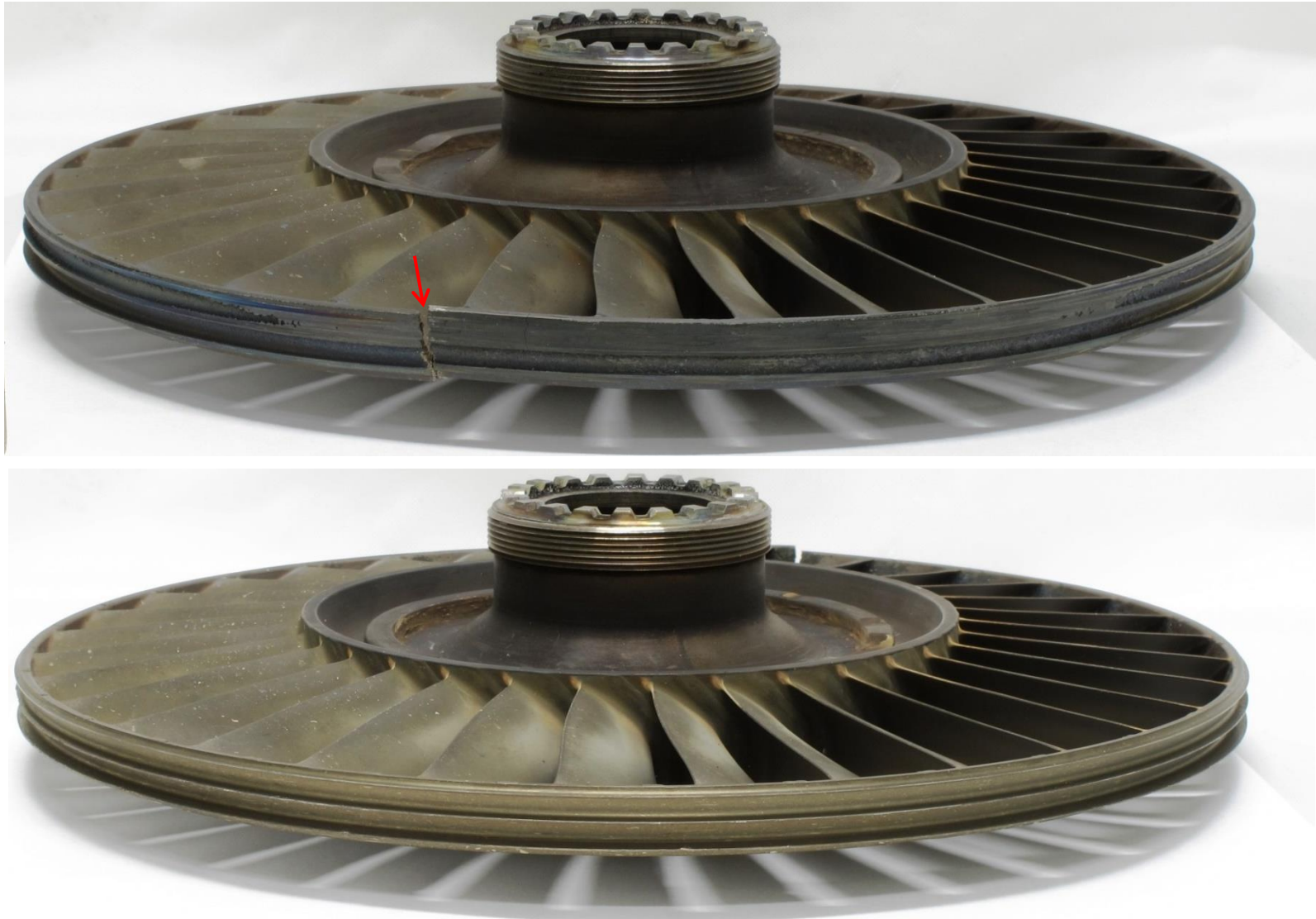
Figure 38. Radial views showing the rub damage to the shroud and knife seals. The shroud band was cracked (red arrow).
