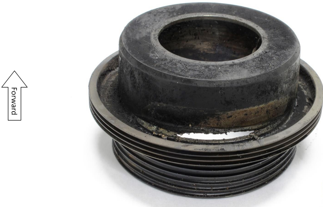
Figure 56. Detailed view showing the rubbed-through area on the third stage power turbine labyrinth seal.
