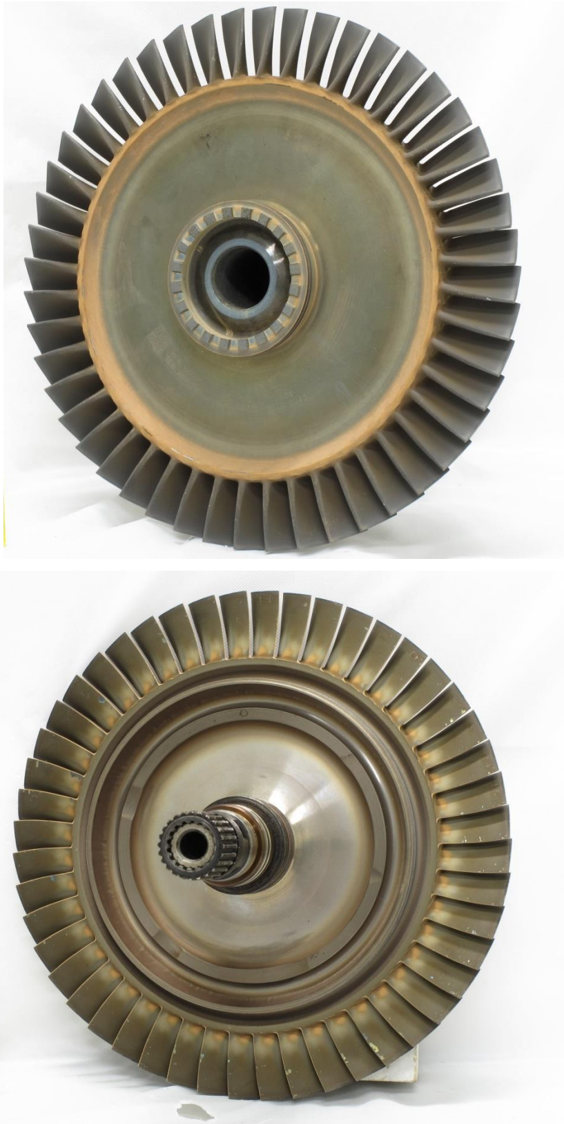
Figure 42. Leading (top) and trailing (bottom) edge side views showing the as-received condition of the second stage turbine wheel. The airfoil trailing edges exhibited impact damage.
