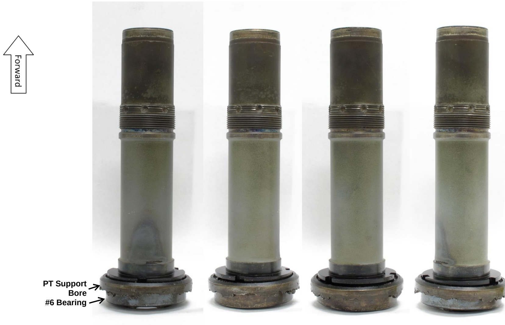
Figure 52. 90° rotated views of the power turbine inner shaft with the No. 6 bearing stuck on the integral inner race. The fractured portion of the PT support bore was retained on the shaft.
