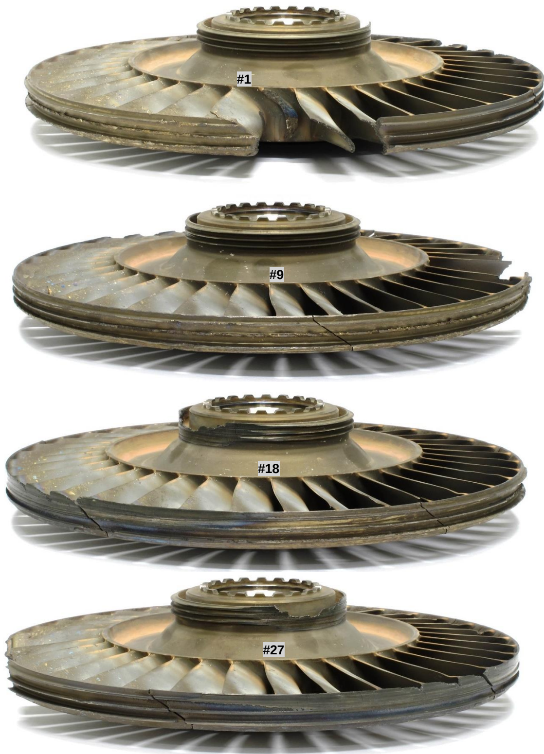
Figure 9. Four views of the third stage turbine wheel showing the extent of the rub damage to the knife seals and shroud. Each image is rotated ~90° from previous in the direction of turbine rotation.
