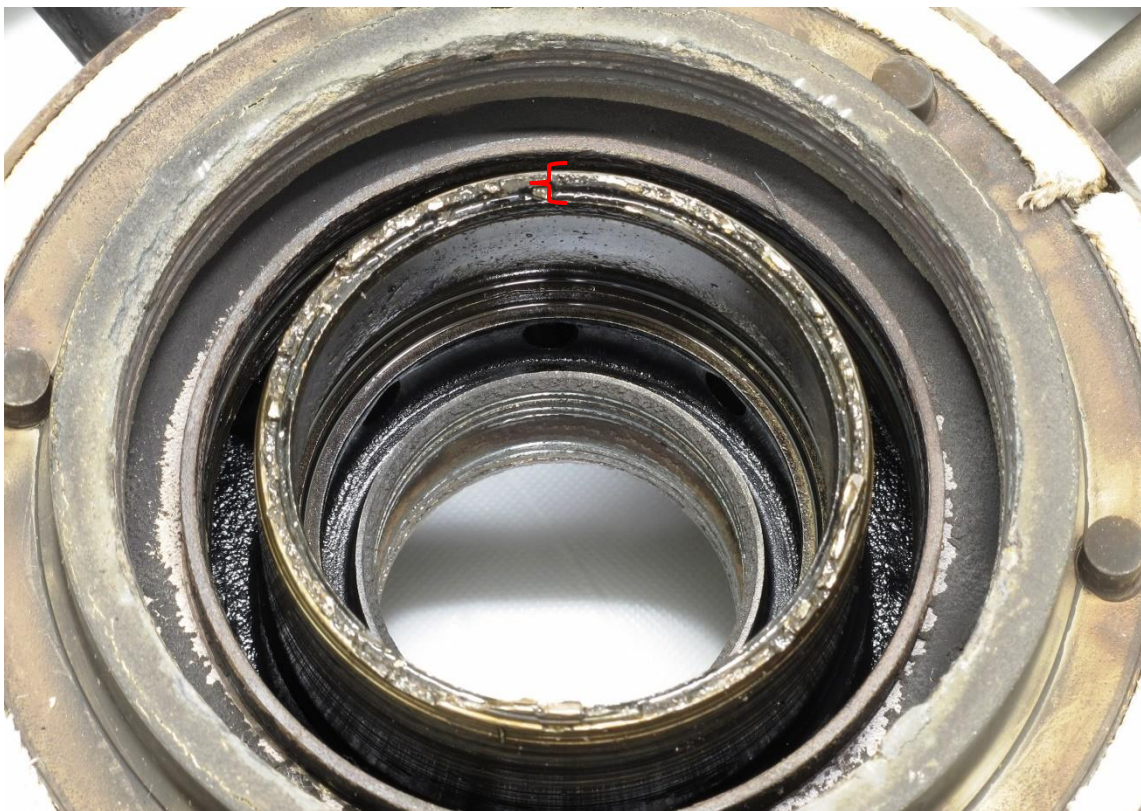
Figure 49. Forward looking aft view of the Nos. 6 and 7 bearing sump in the power turbine support. The bore of the sump was fractured circumferentially at the forward end (red brace).
