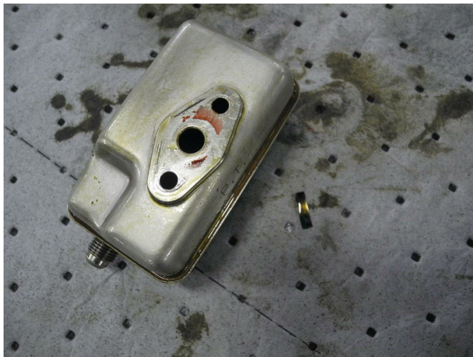
Photo 6 - #6 and #7 Bearing Oil Sump Can
