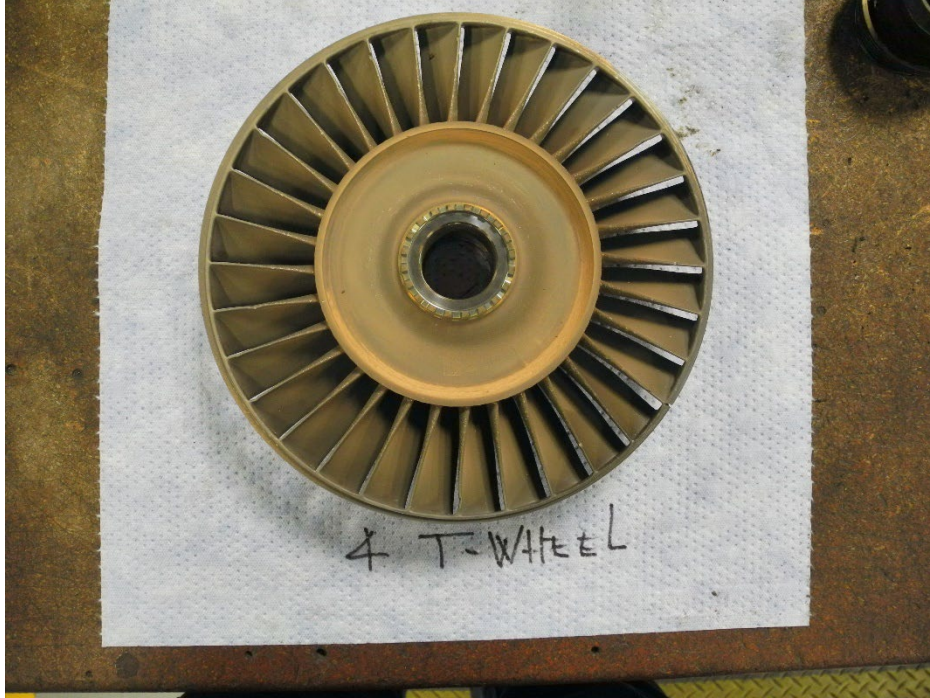
Photo 21 - 4 th Stage Turbine Wheel – Upstream Side
