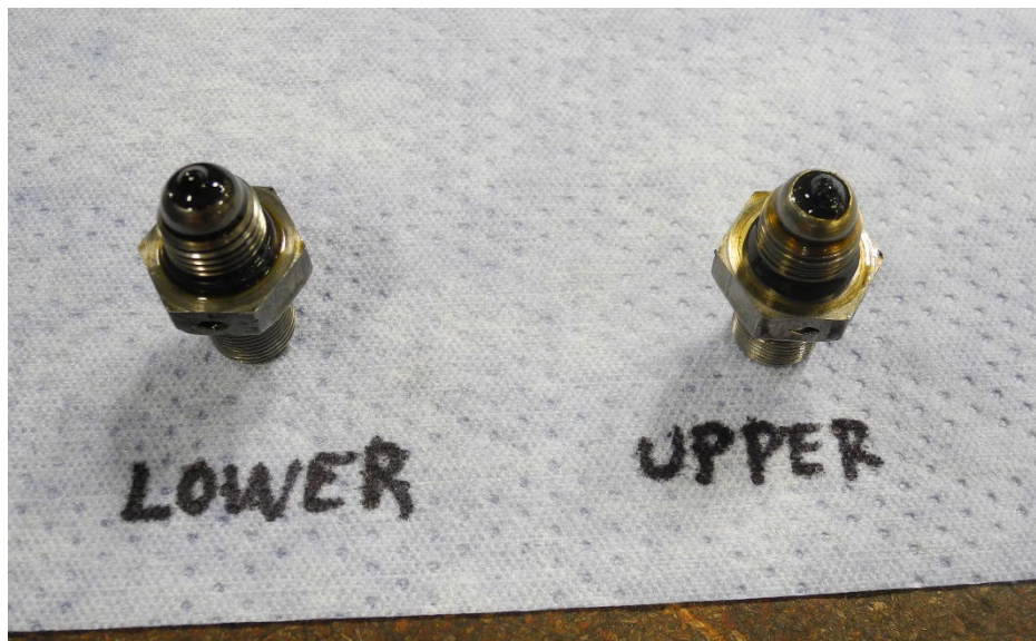
Photo 5 – Chip Detectors - Clean
