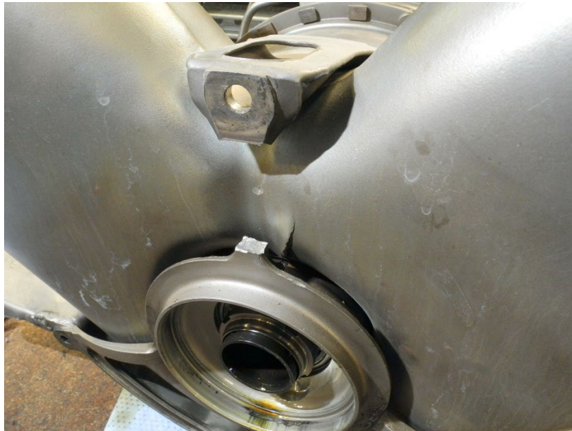
Photo 24 - Exhaust Collector Support Strut and Duct Fracture
