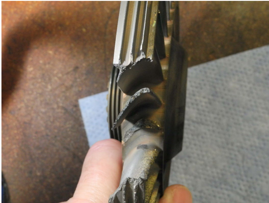
Photo 18 - Adjacent Blade Fracture Detail
