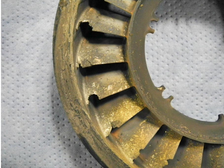
Photo 15 - 3 rd Stage Turbine Nozzle – Downstream Face - Detail
