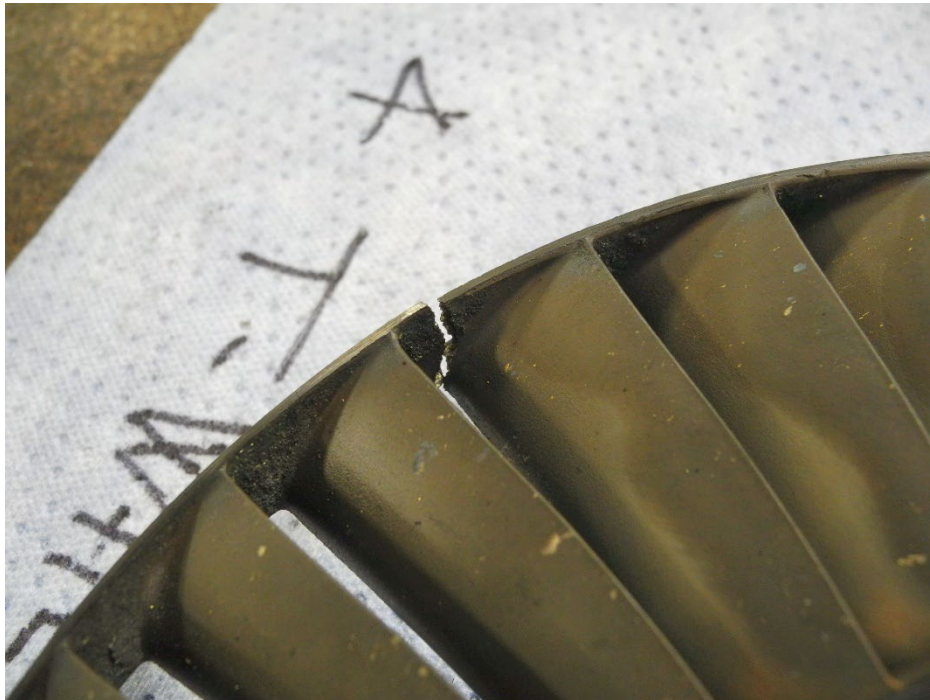
Photo 22 - 4 th Stage Turbine Wheel – Shroud Fracture
