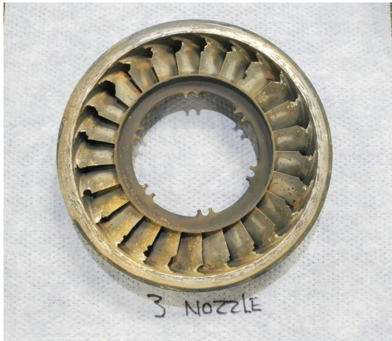
Photo 14 - 3 rd Stage Turbine Nozzle – Downstream Face
