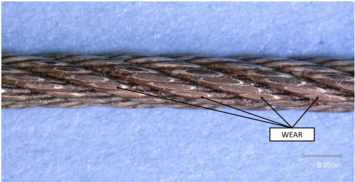
Figure 2: Magnified view showing external wear to the individual wires from the section of cable identified in figure 1. Arrows indicating several locations of features consistent with wear.
