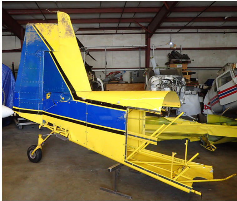
Aft Fuselage Wreckage
