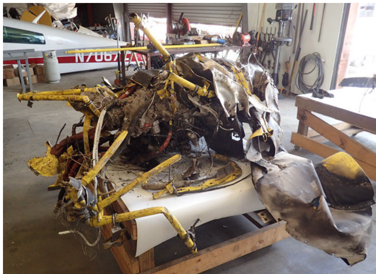
Engine Mount Wreckage (Right Side)
