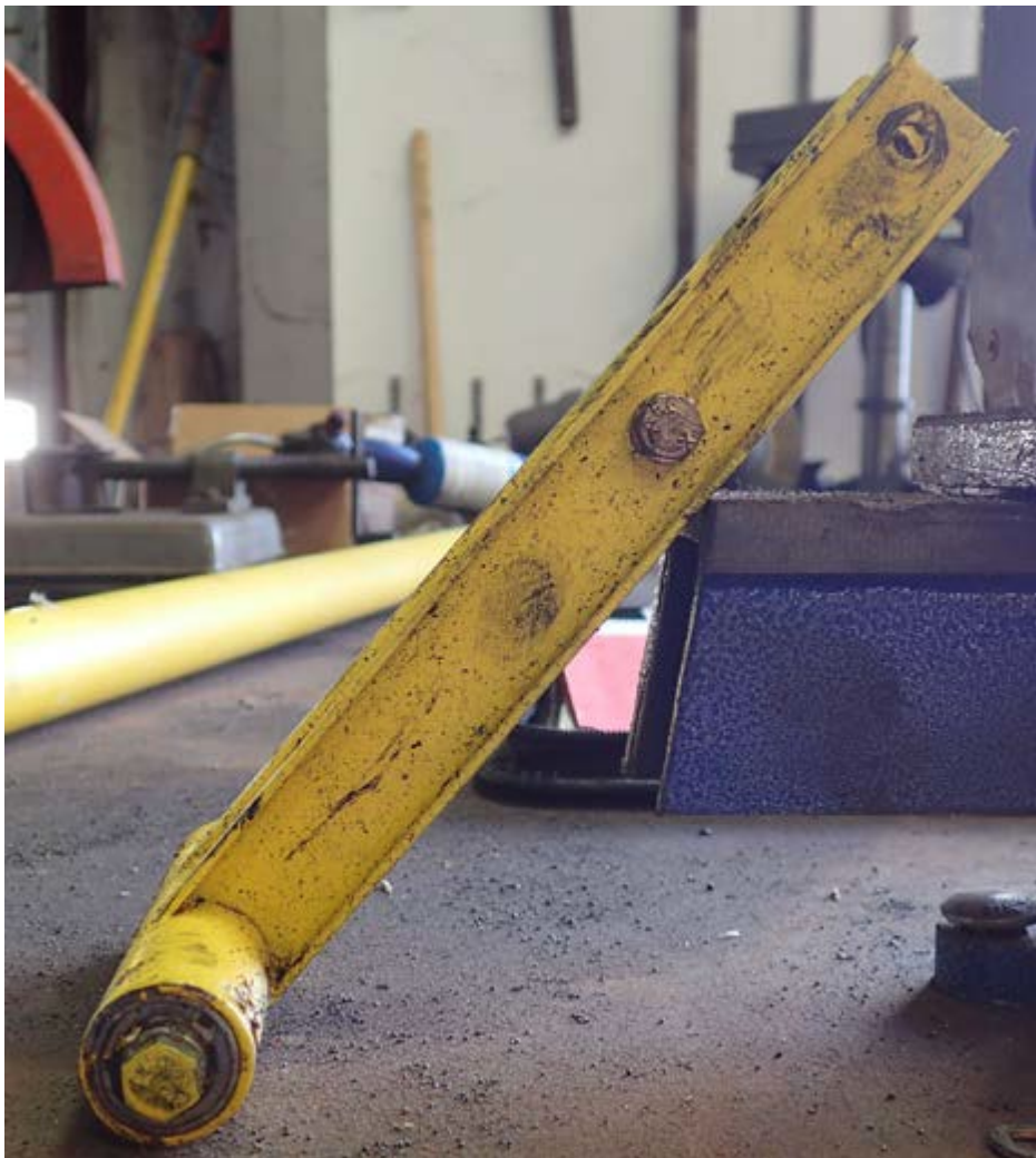
Photo 4 - Forward Elevator Idler (Courtesy of Air Tractor)
