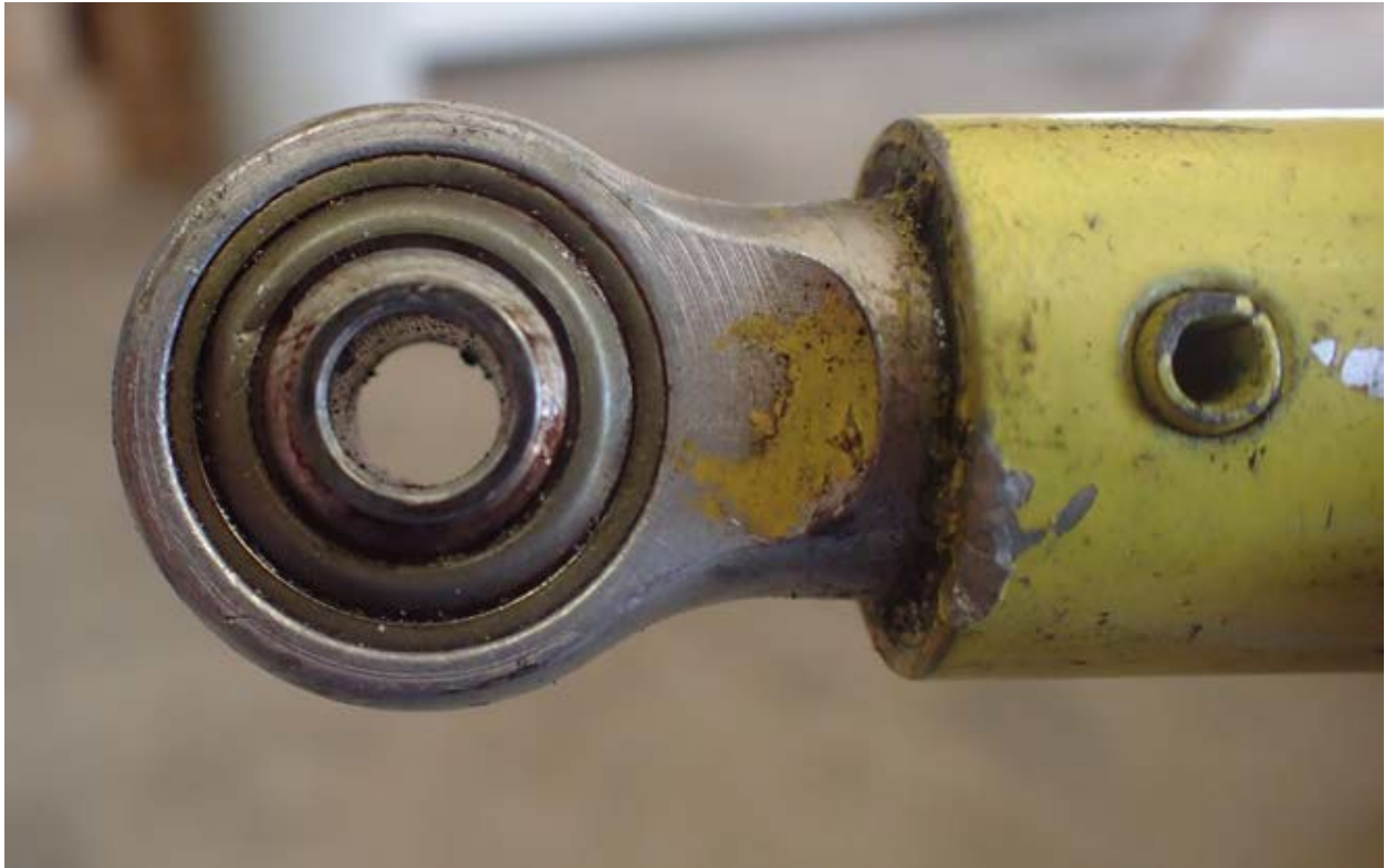
Photo 5 - Forward Rod End Bearing of Elevator Pushrod (Courtesy of Air Tractor)
