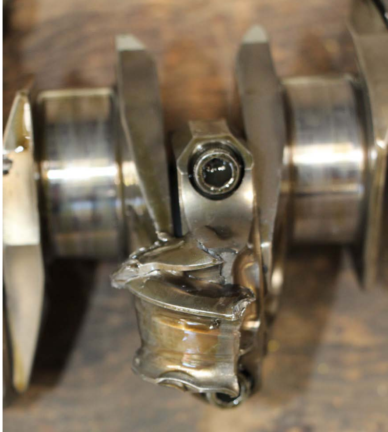
Photograph 11: Portion of Cylinder No. 5 Connecting Rod
