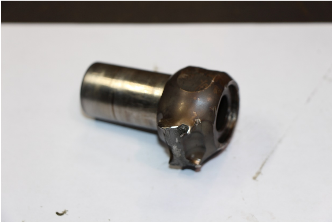
Photograph 7: Cylinder No. 5 Piston Wrist Pin
