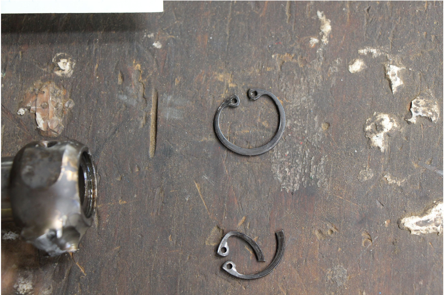
Photo 3 – View of Cylinder no. 5 Piston Circlips (Courtesy of NTSB)
