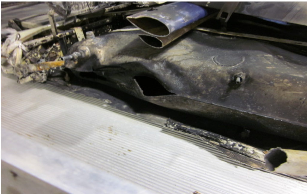
Right fuel tank breach, inboard side of tank.
