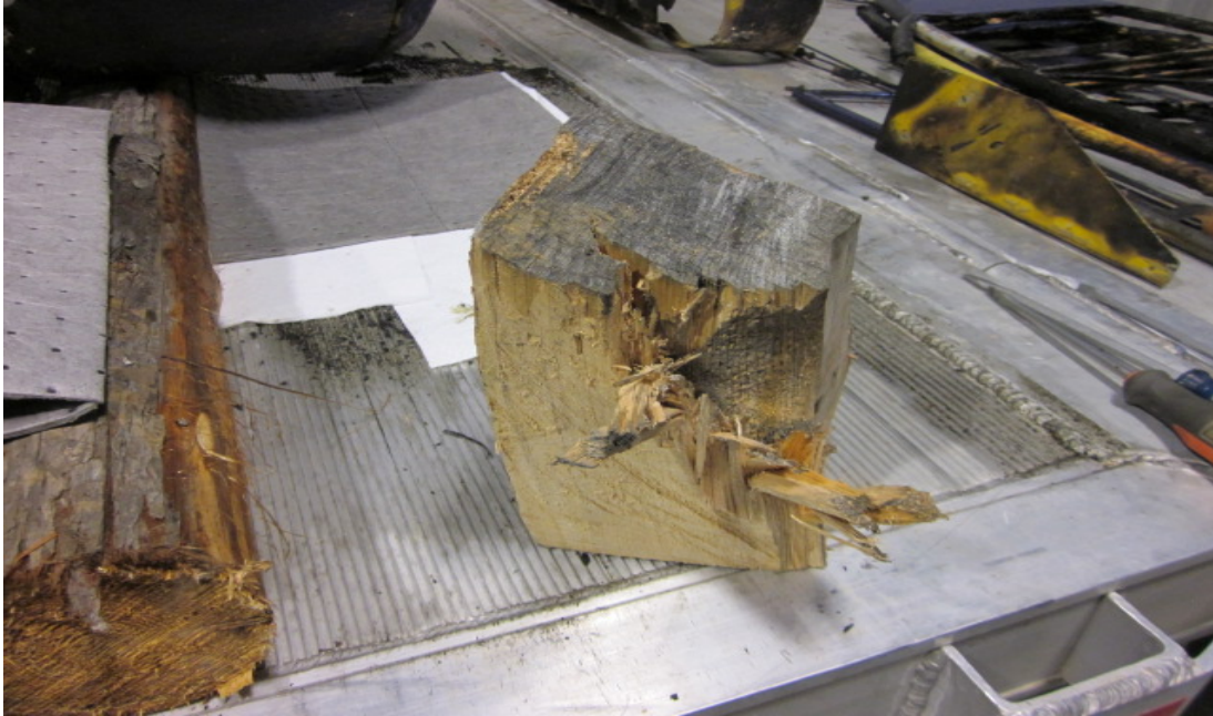
Stump section, Propeller strike.
