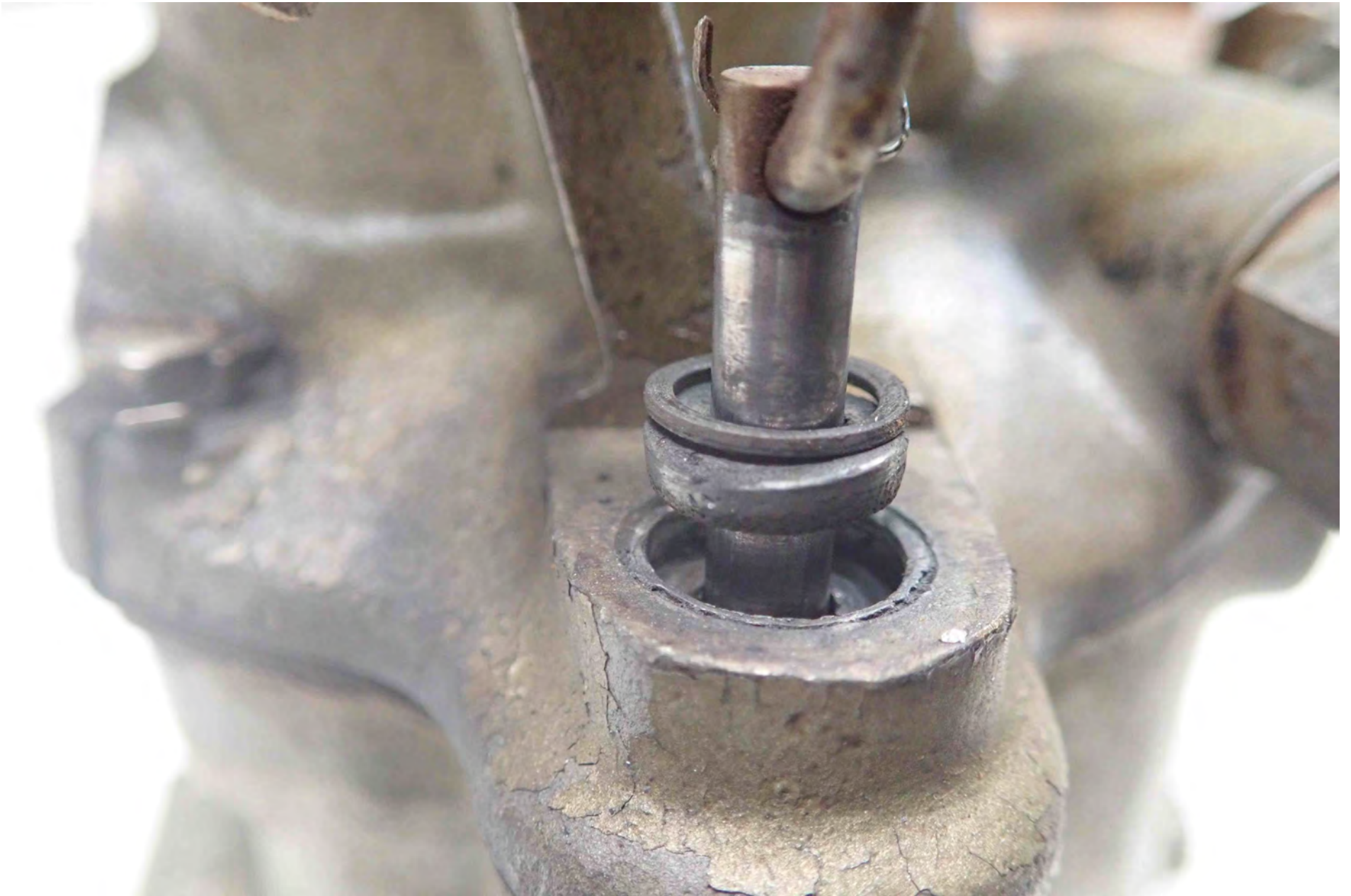
Photo 6 – Loose Accelerator Pump Packing
