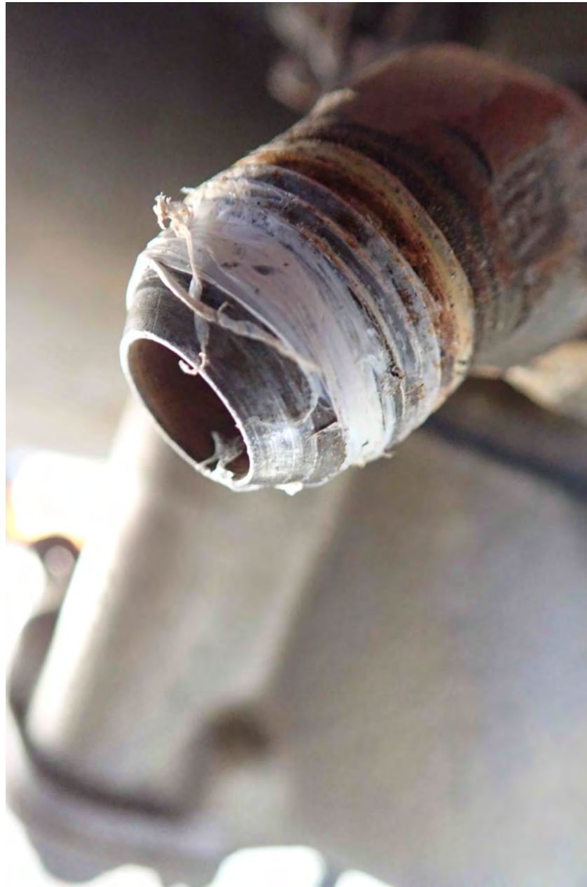
Photo 5 – Teflon Tape on Carburetor Fuel Inlet Fitting
