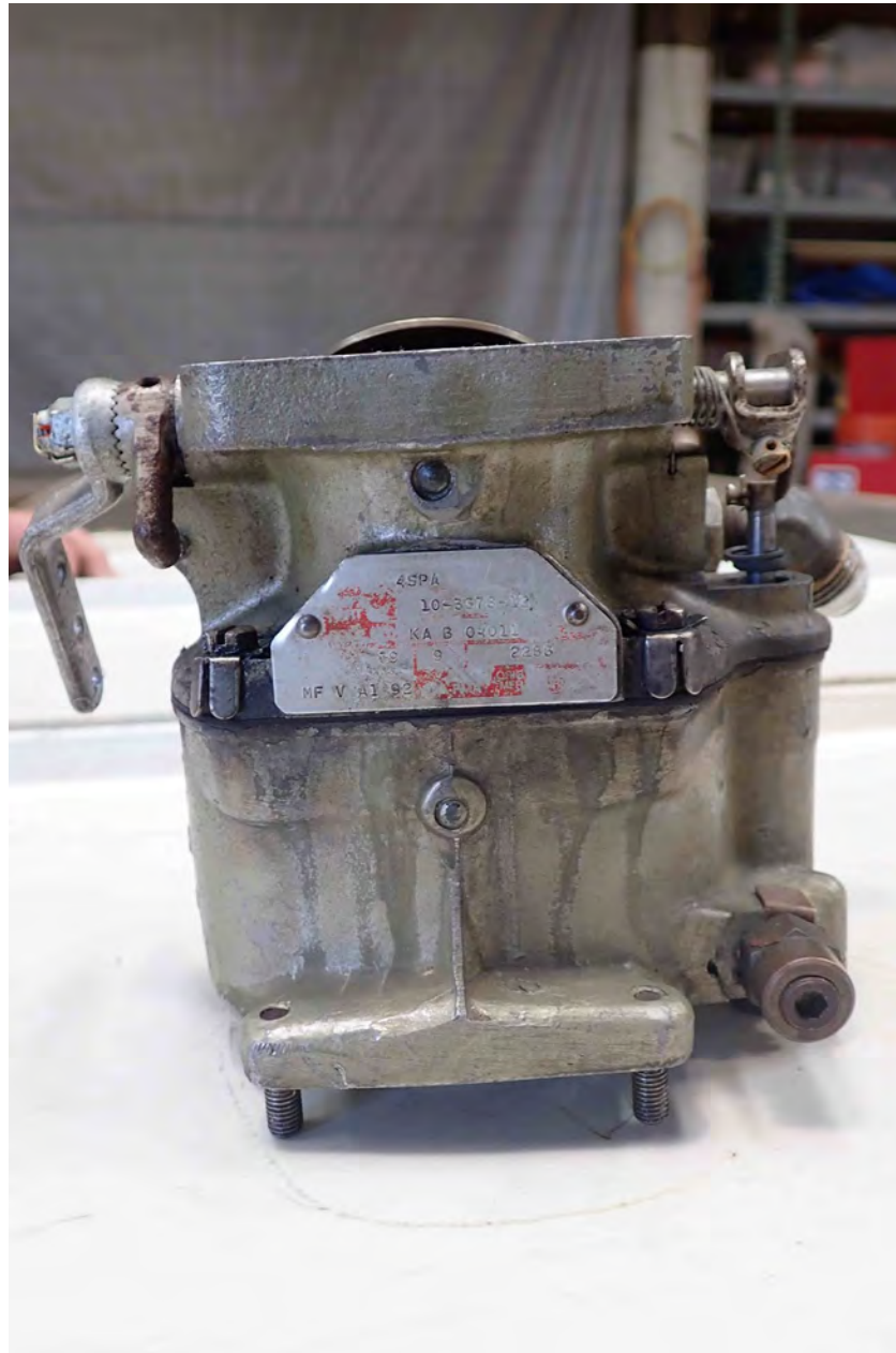
Photo 7 – Fuel Leak at Body-to-Bowl Join
