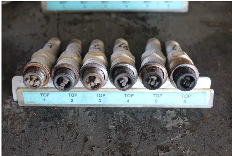
Figure 2 - top spark plugs
