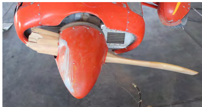
Figure 4 - photo of propeller and spinner as received
