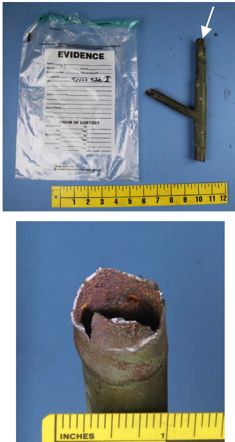
Figure 1: The top photo shows an overall view of truss tube I. The white arrow points to the viewing perspective in the close-up shown in the bottom photo.
