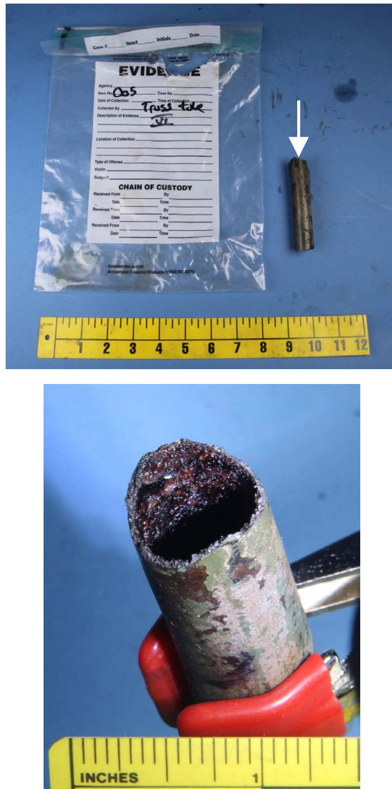
Figure 6: The top photo shows an overall view of truss tube VI. The white arrow points to the viewing perspective in the close-up shown in the bottom photo.
