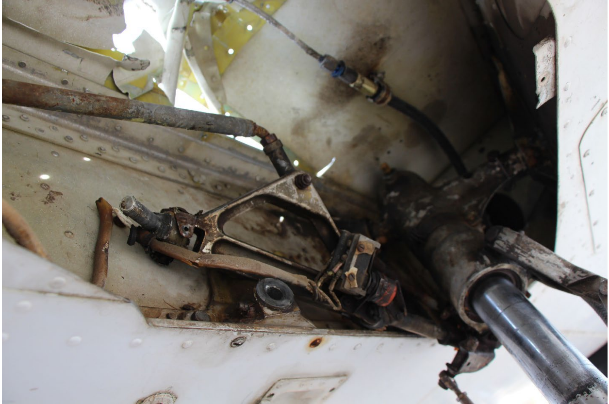
Photograph 9: Right Main Landing Gear Strut and Assembly (NTSB)
