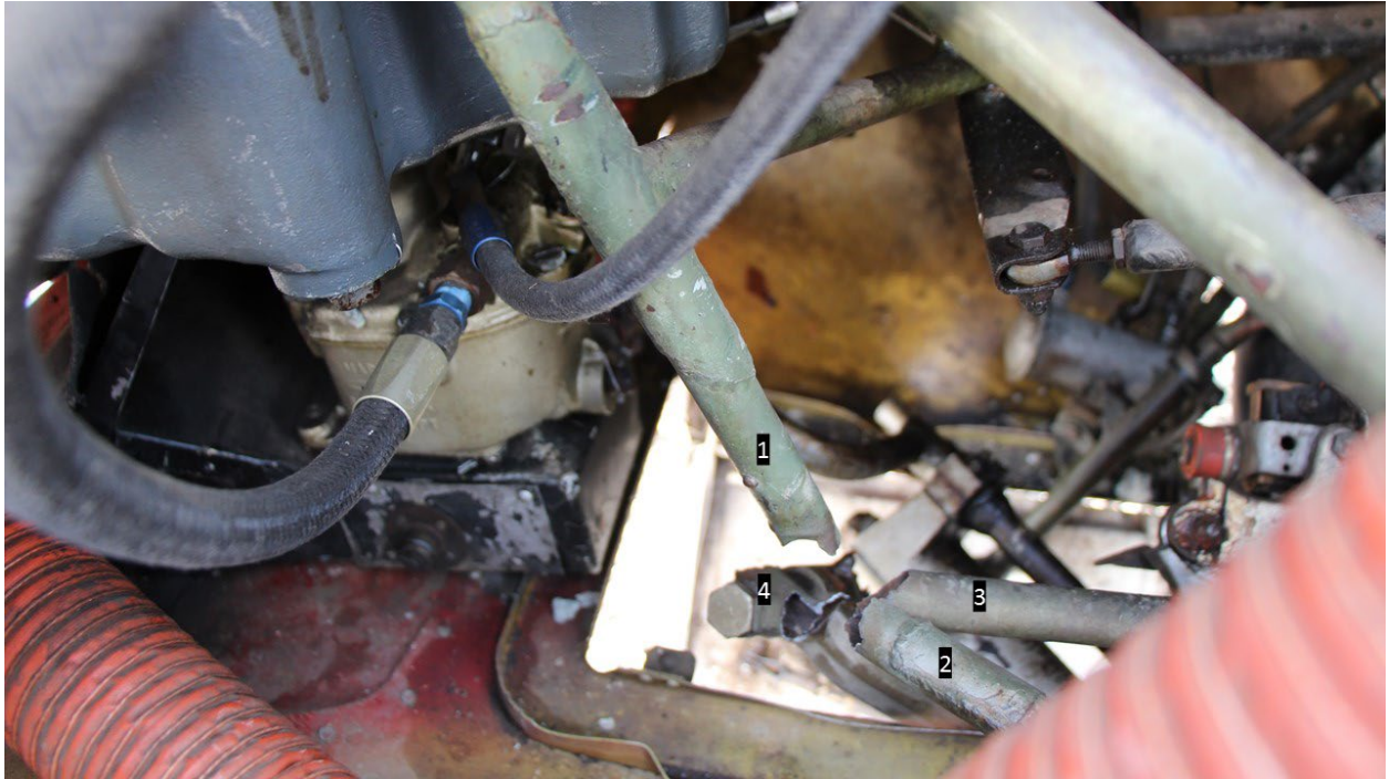
Photograph 3: LH Engine Mount Tubes and NLG Trunnion (Nos. 1 – 4) (NTSB)
