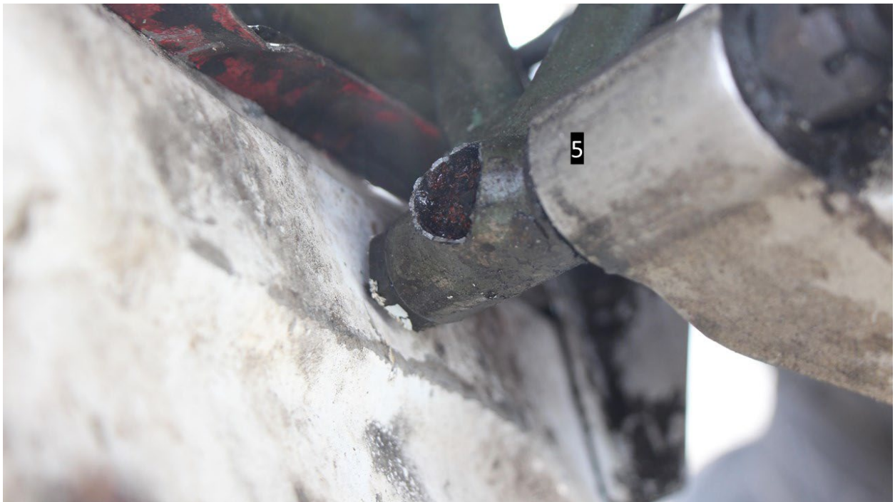
Photograph 4: RH Engine Mount and NLG Trunnion (No. 5) (NTSB)
