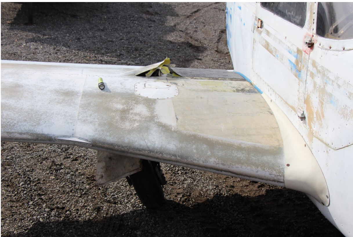
Photograph 8: Right Wing with Protrusion Through Top Skin (NTSB)
