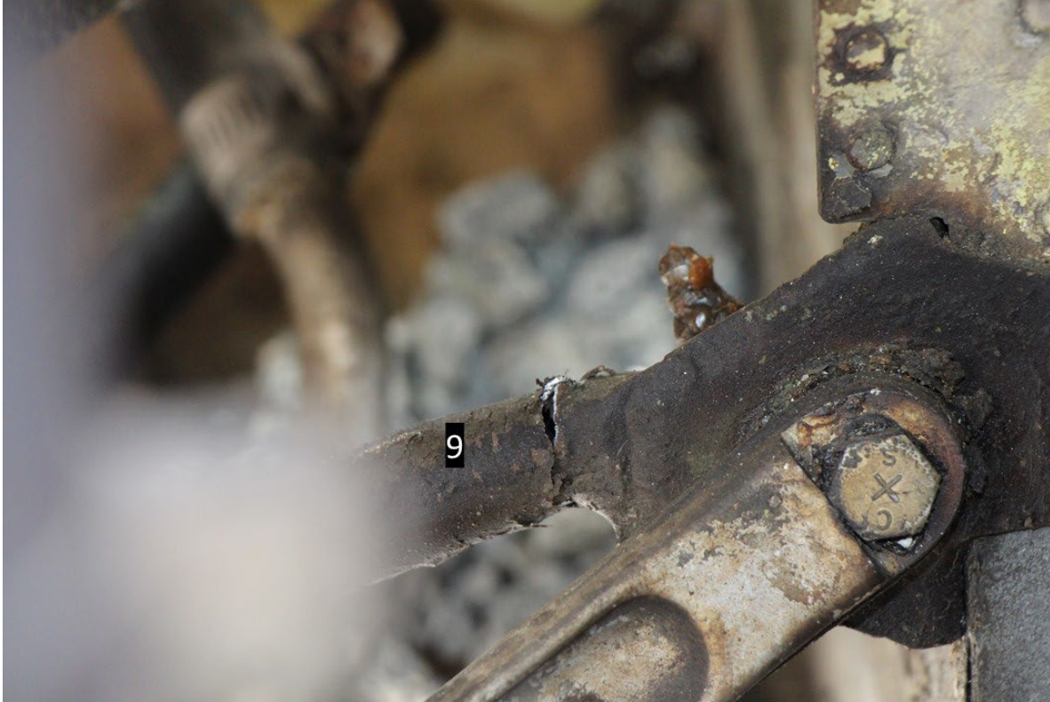
Photograph 7: RH Engine Mount Tube at Engine Firewall; No. 6 (NTSB)
