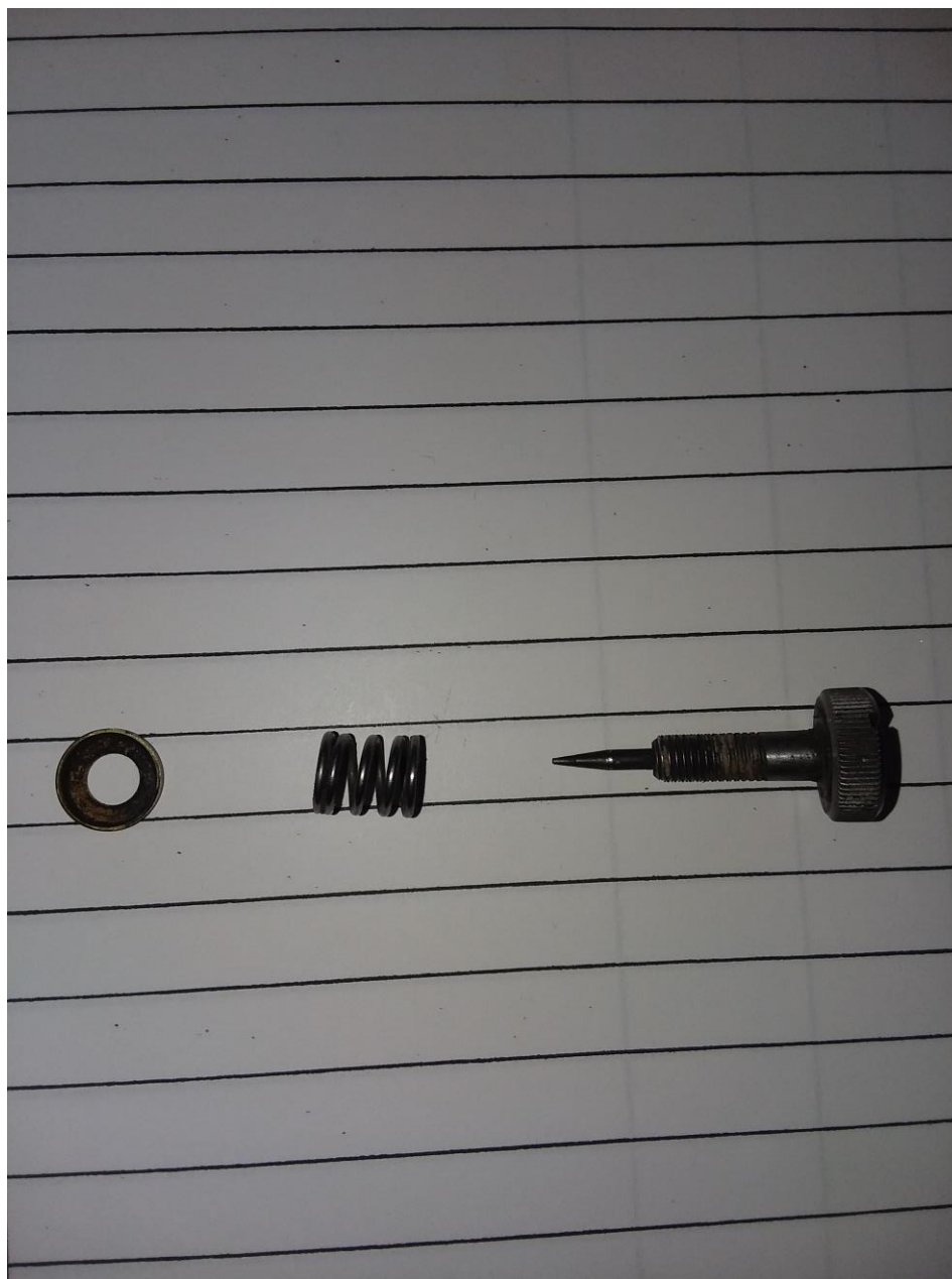
Photo 4 - Idle Mixture Adjustment Screw and Spring Assembly (Courtesy of the airplane owner)
