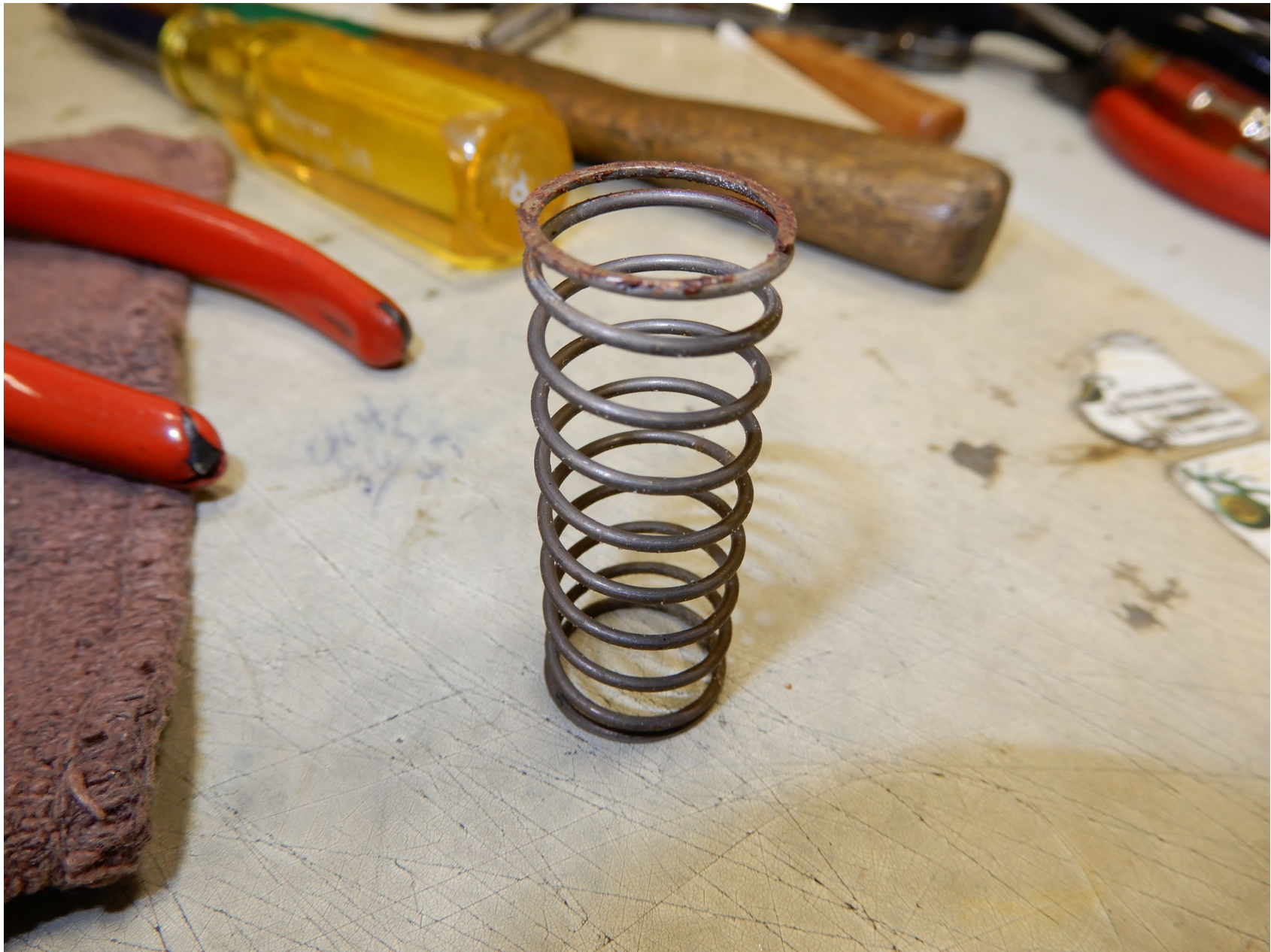
Photo 7 – Bleed valve spring, showing corrosion on top of spring.
