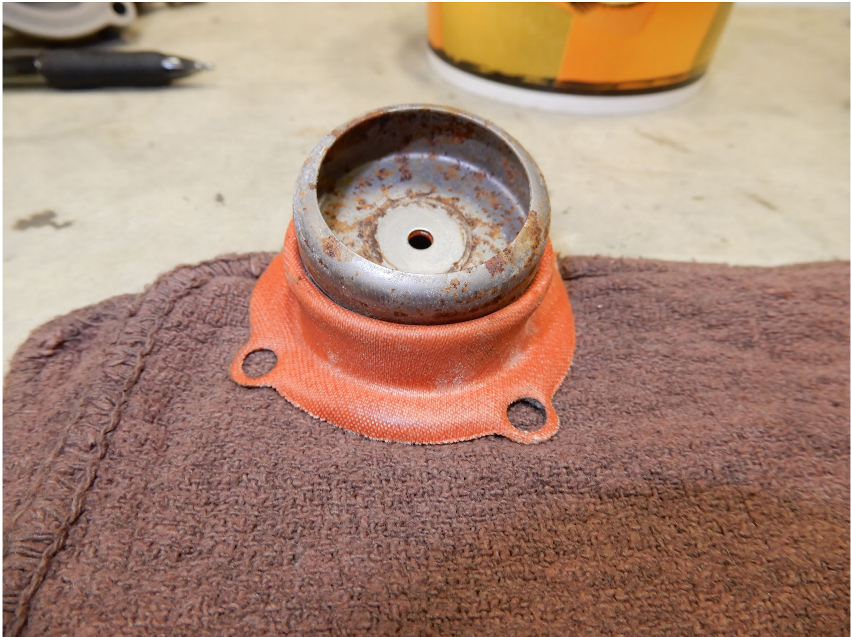
Photo 8 – Bleed valve bellows, showing corrosion.
