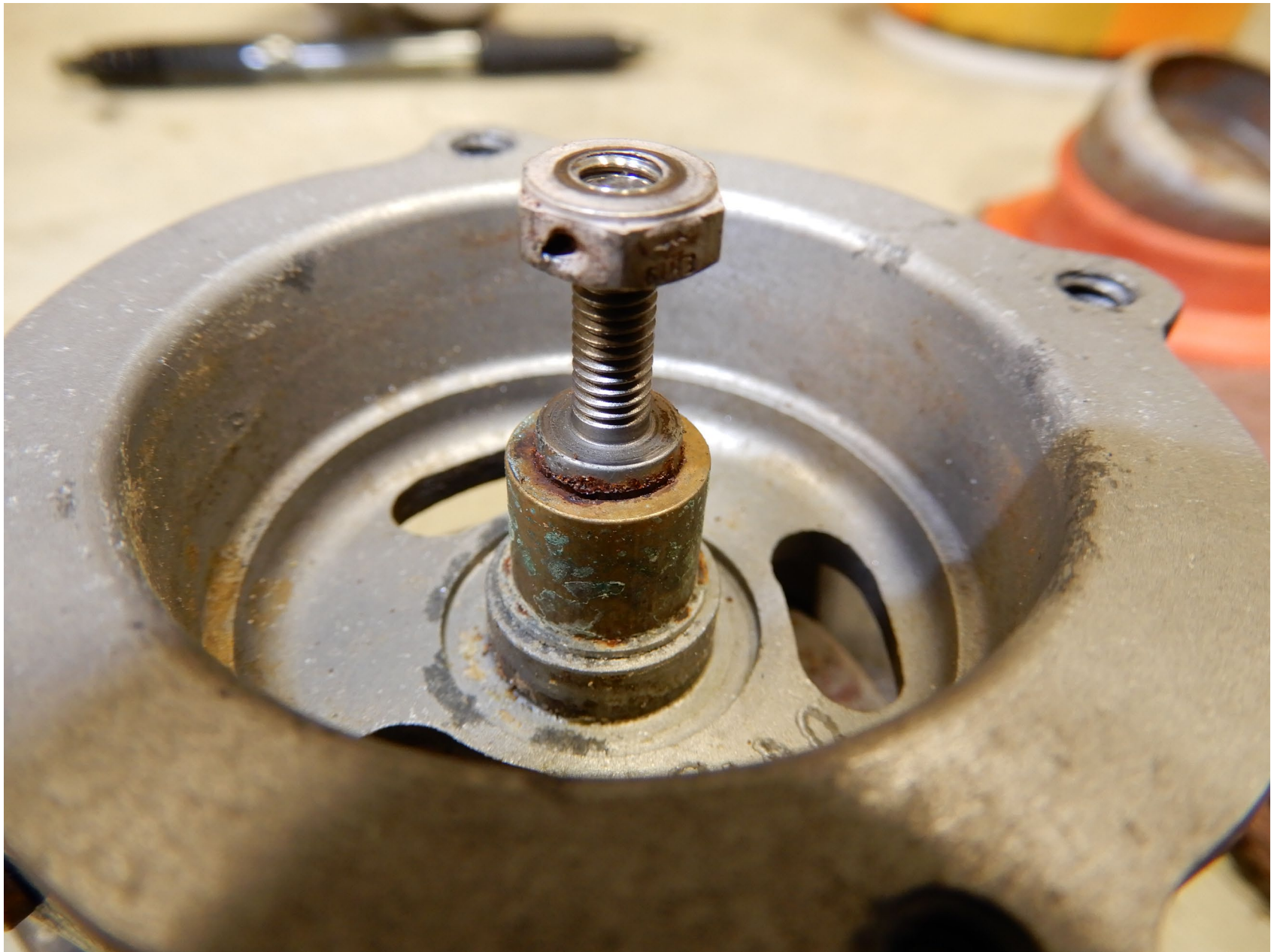
Photo 5 – Accident compressor bleed valve assembly, showing corrosion on valve and guide.
