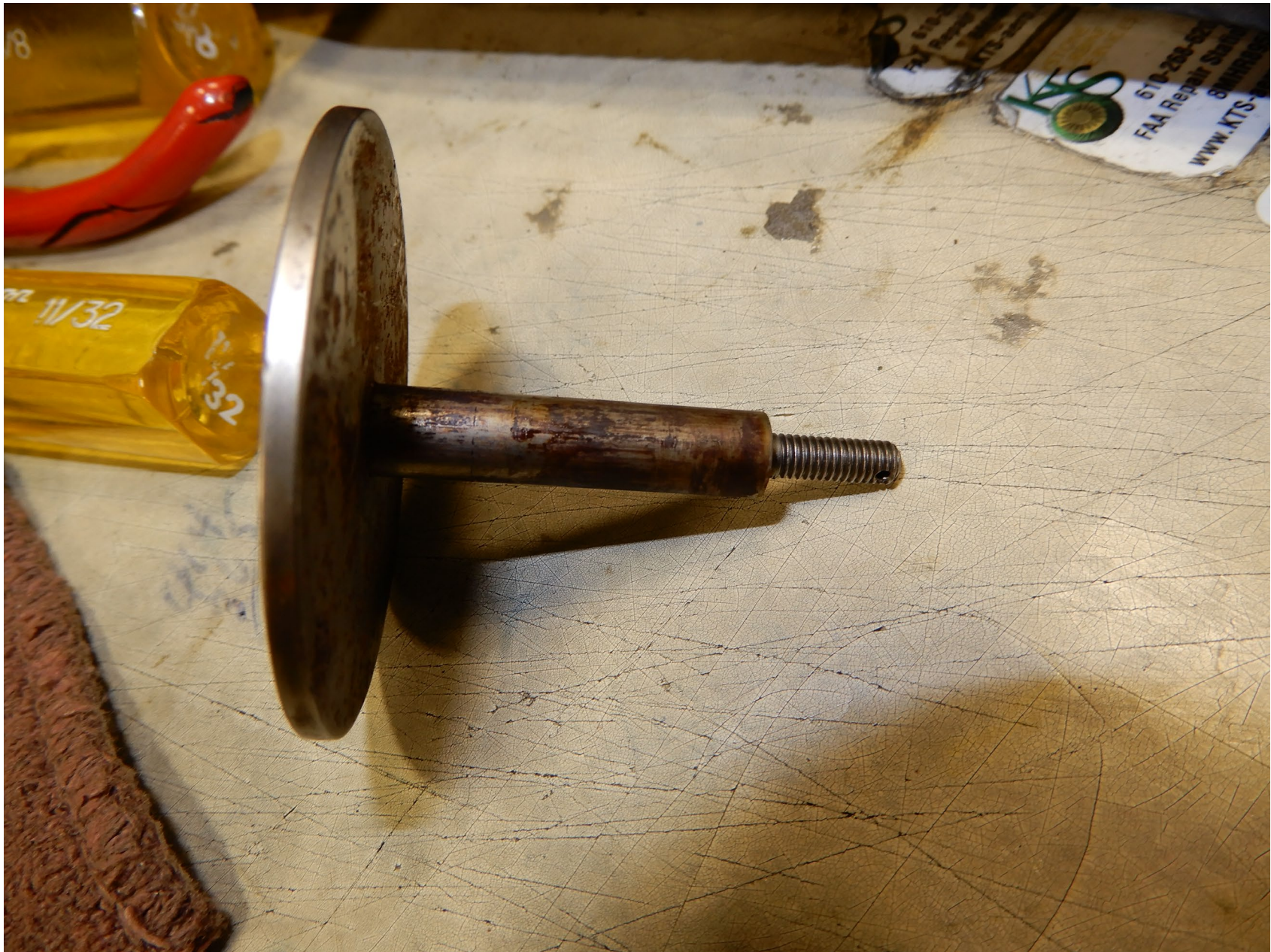
Photo 6 – Accident compressor bleed valve, showing corrosion build up on valve stem.
