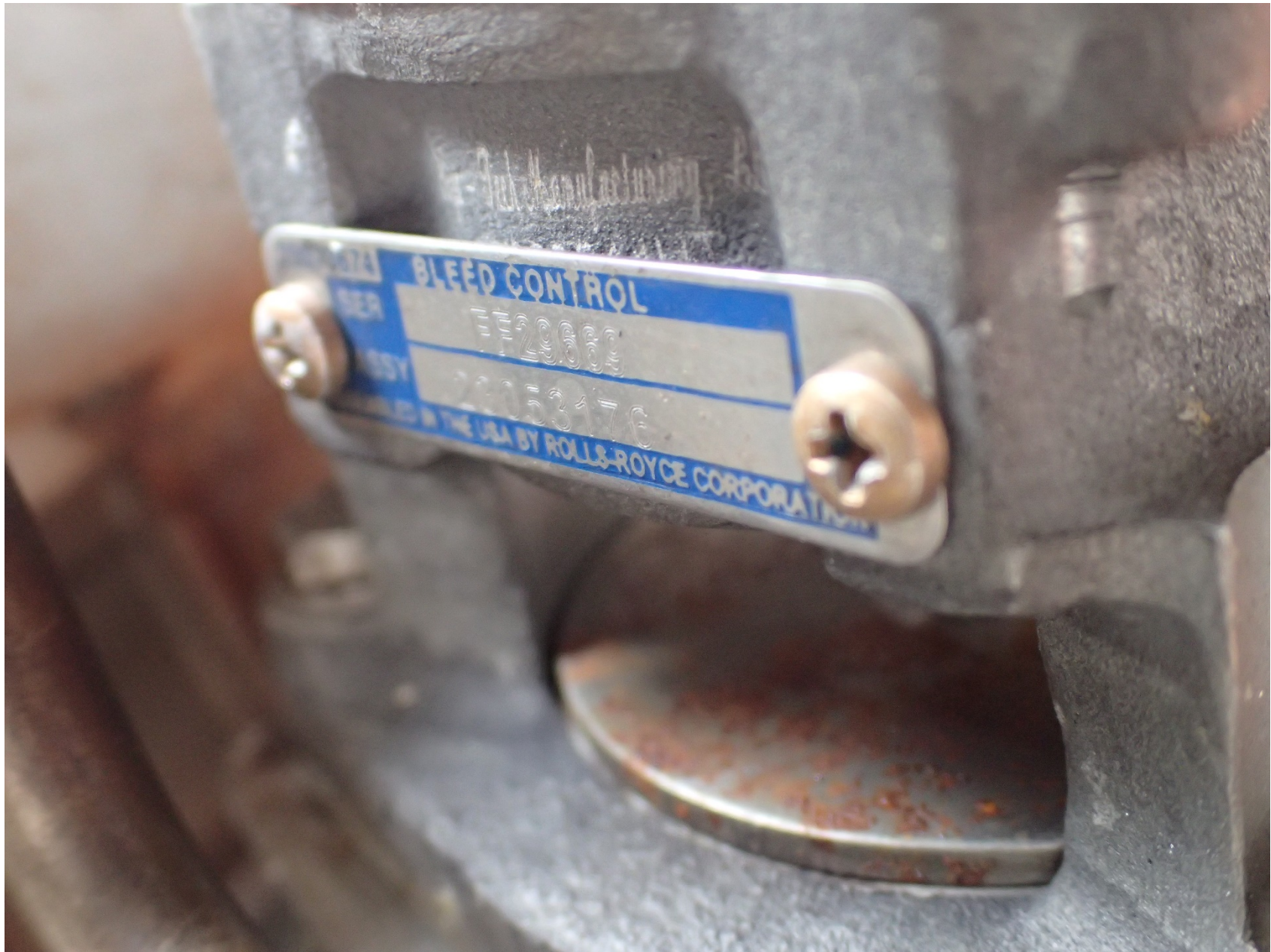
Photo 4 - Bleed valve assembly mounted on engine showing valve in the closed position.
