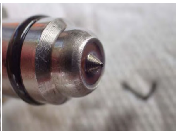
Lower Chip Detector
