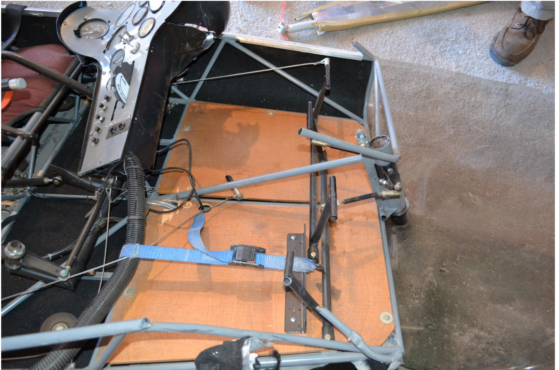
Photo 11 – Cabin Floor and Ballast Tiedown Area
