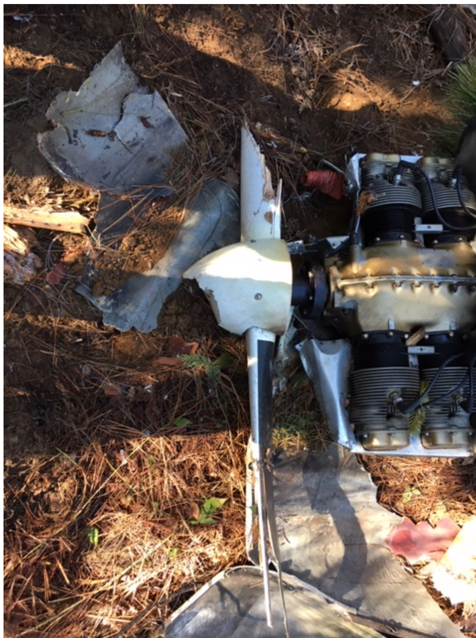
Photo 4 – view of engine and propeller at rest upright at accident site (courtesy of Federal Aviation Administration)
