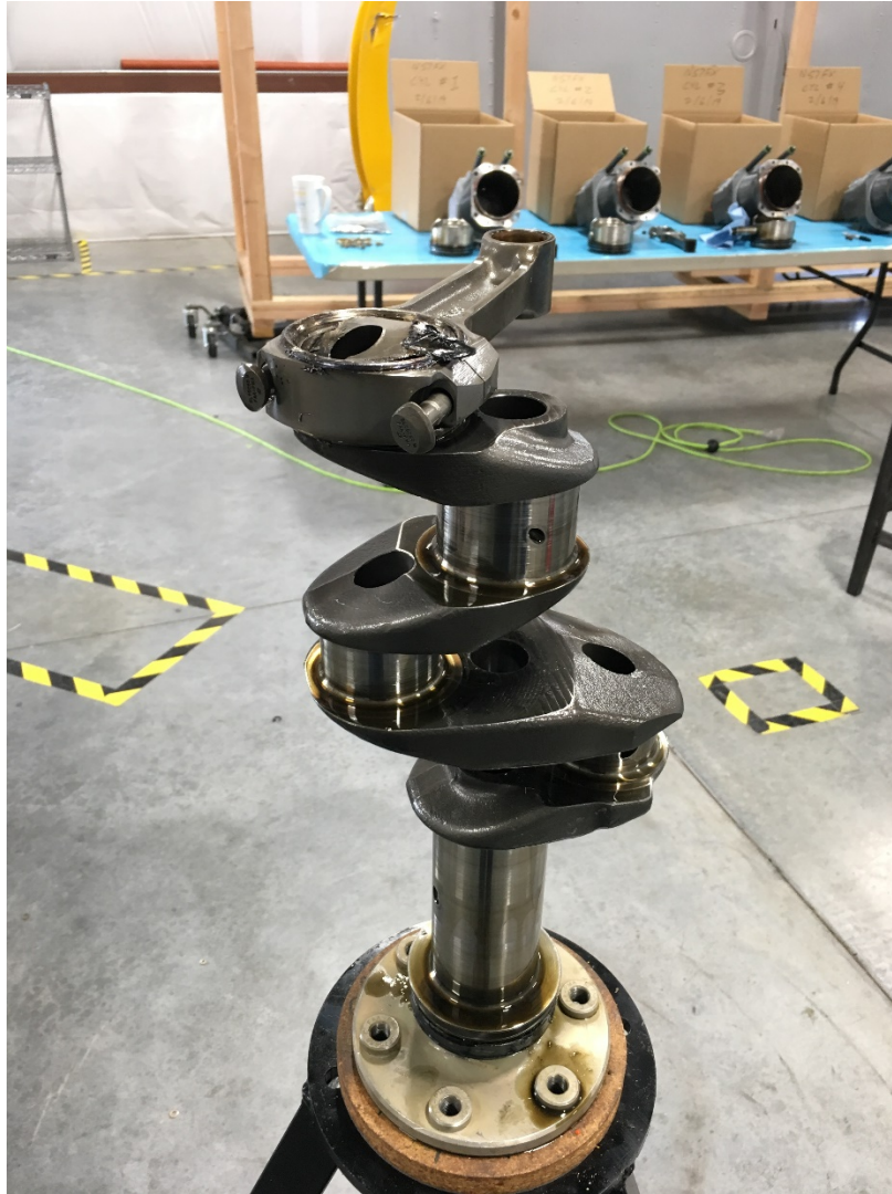
Figure 6 Fractured Crankshaft FWD Section
