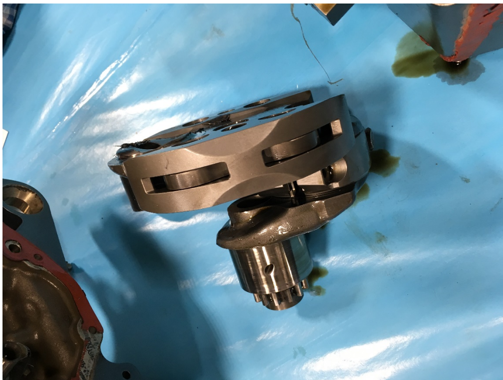
Figure 7 Fractured Crankshaft AFT Section
