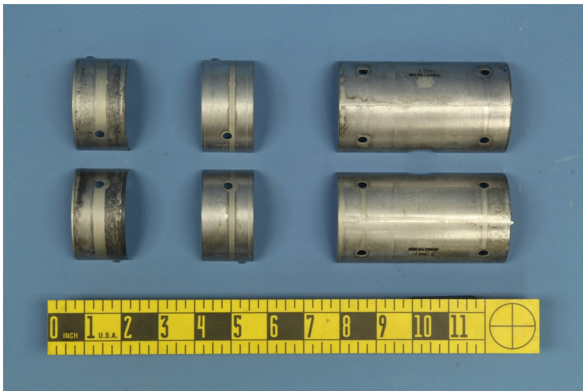
Figure 3: Images of the bearing shells: a) bearing surfaces and b) backsides in contact with the crankcase saddles.
