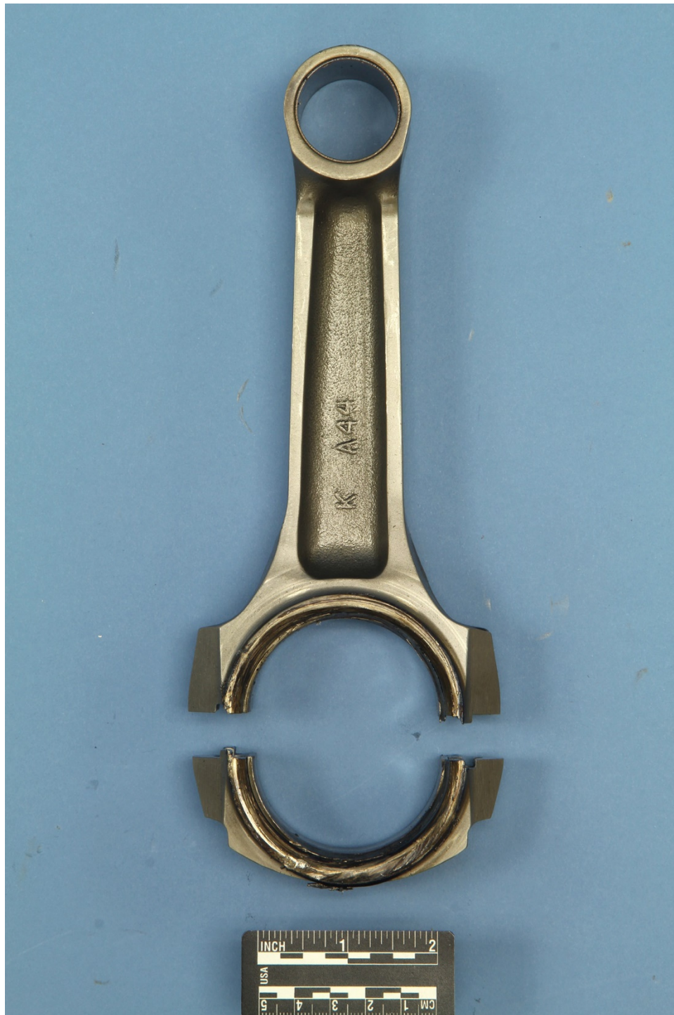
Figure 5: Image of the number 3 connecting rod and endcap after removal from the crankshaft.
