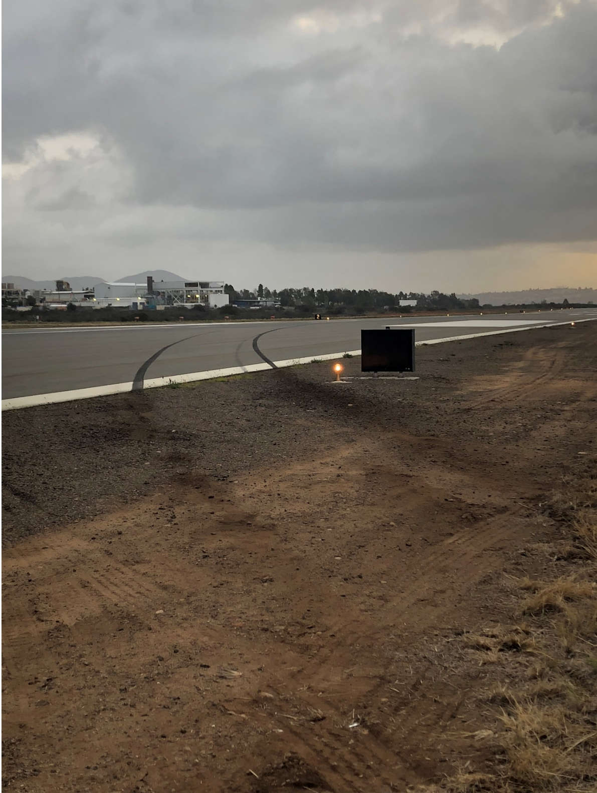
Skid Marks on the Runway (Photo provided by Gibbs Aviation)
