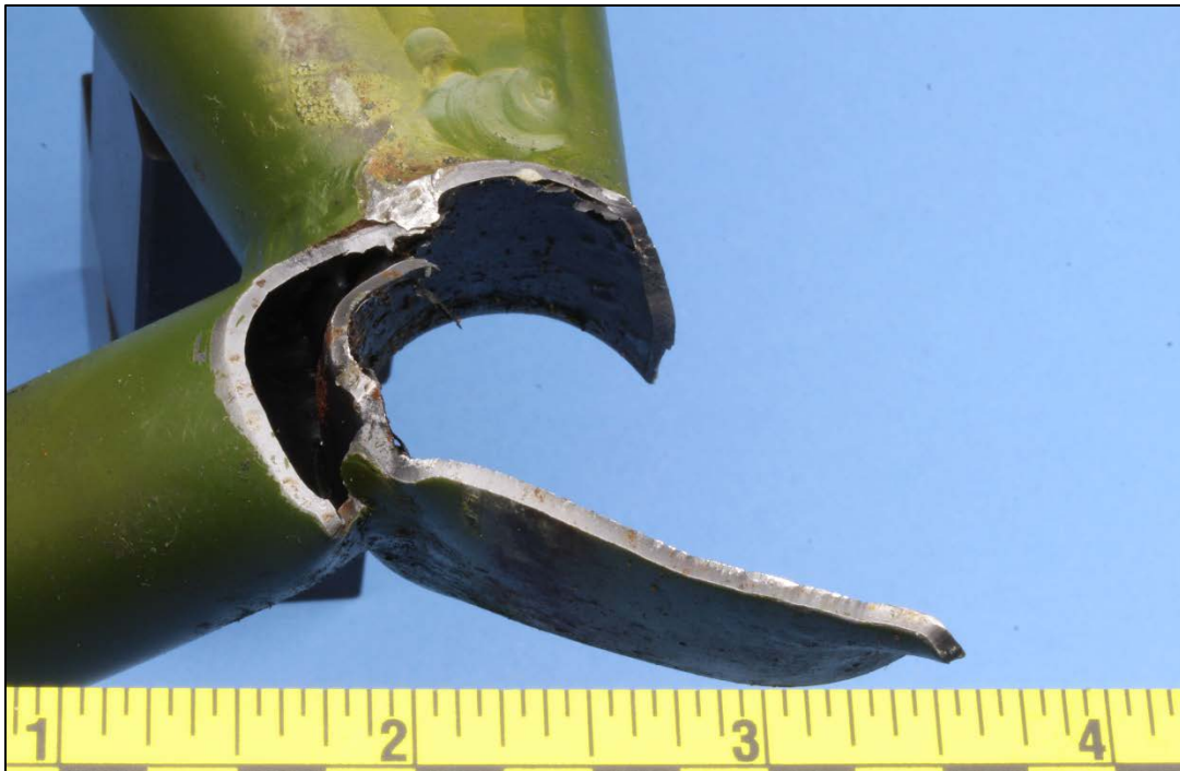
Figure 2. Close view of the fracture at the right nose landing gear actuator attachment foot.
