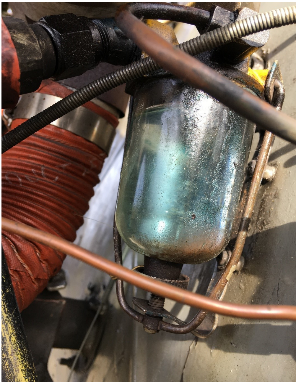
Photo 5 – Fuel System Gascolator (Courtesy of Federal Aviation Administration)
