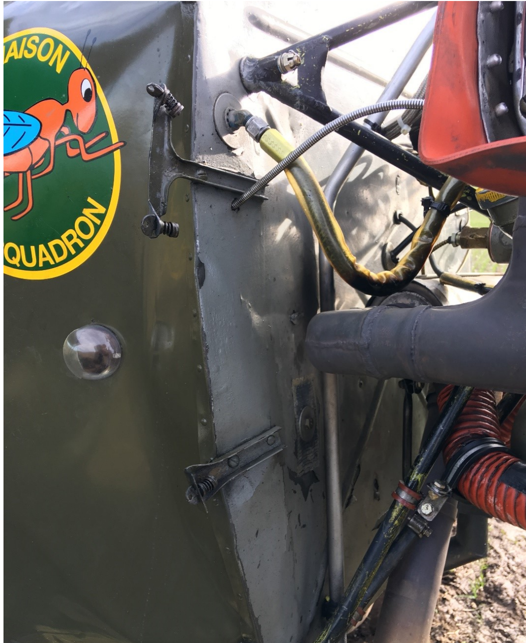
Photo 3 – View of Engine Firewall (Courtesy of Federal Aviation Administration)
