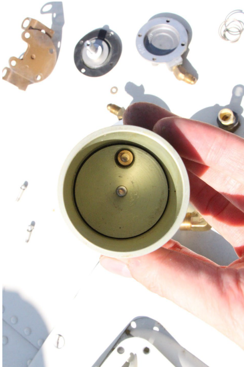
Photograph 4: Gascolator Fuel Bowl
