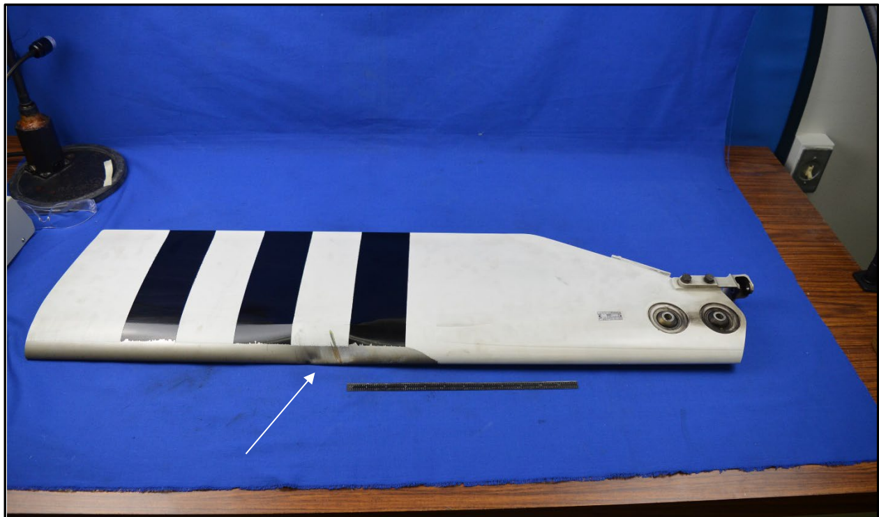
Figure 2: Tail rotor blade (1) as received, with dent near mid-span of leading edge.
