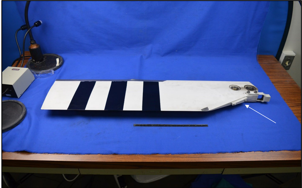
Figure 1: Tail rotor blade (1) as received, with root enclosure and attached weights intact.
