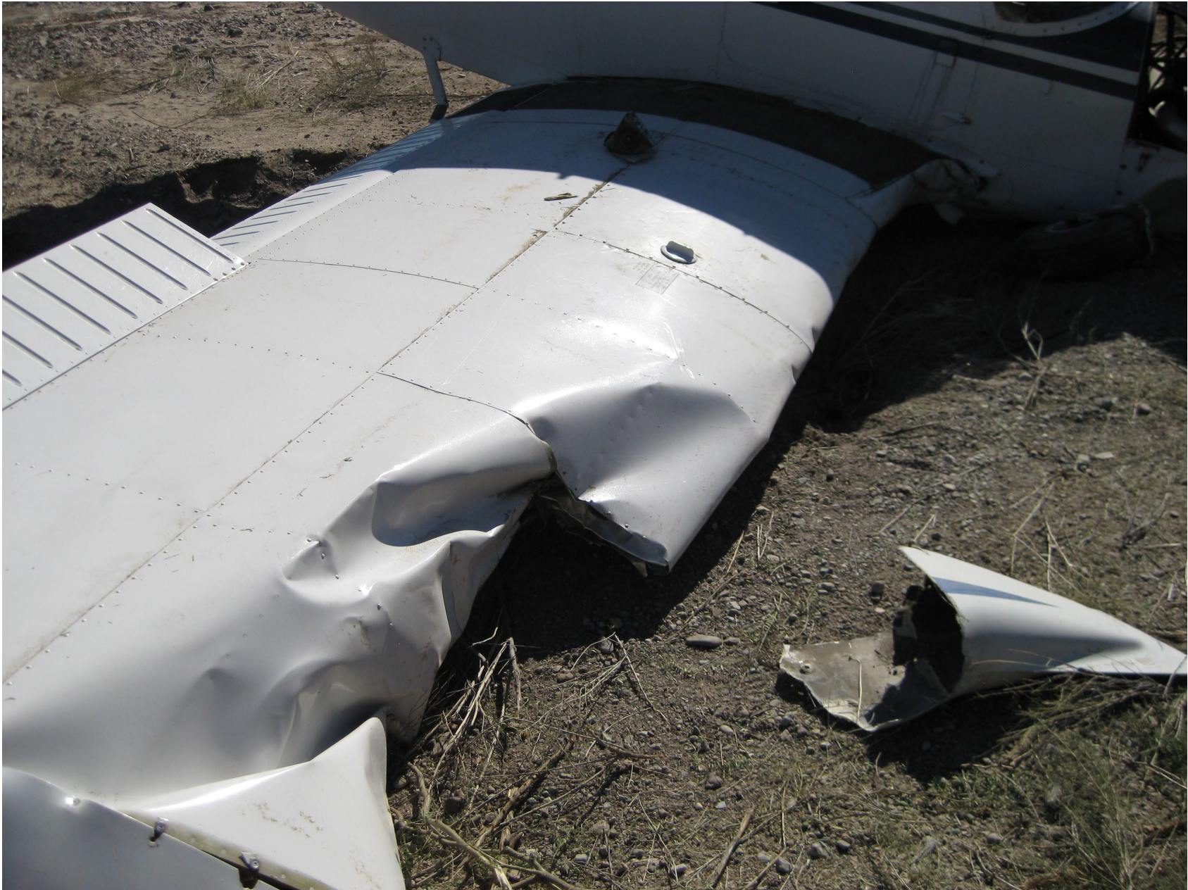
Photo 3 – Close-up View of Damaged Right Wing (Photo Courtesy of FAA)
