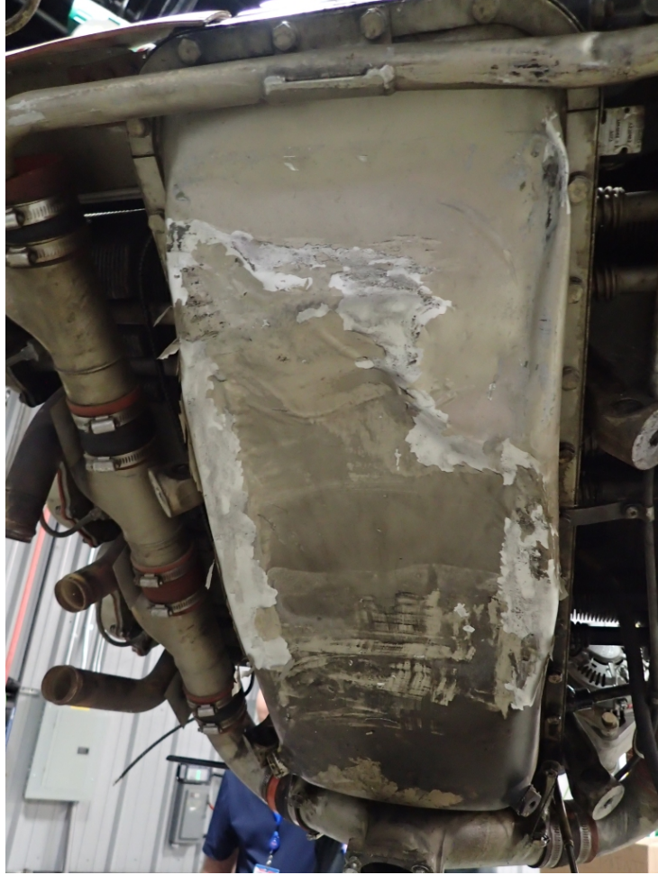
Figure 10 - Damaged Oil Sump
