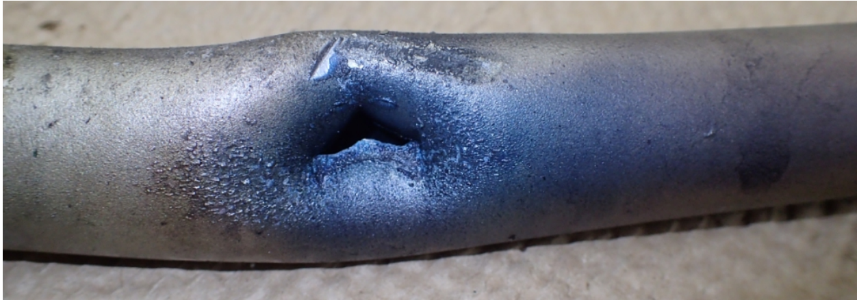
Figure 13 - Puncture in Balance Tube
