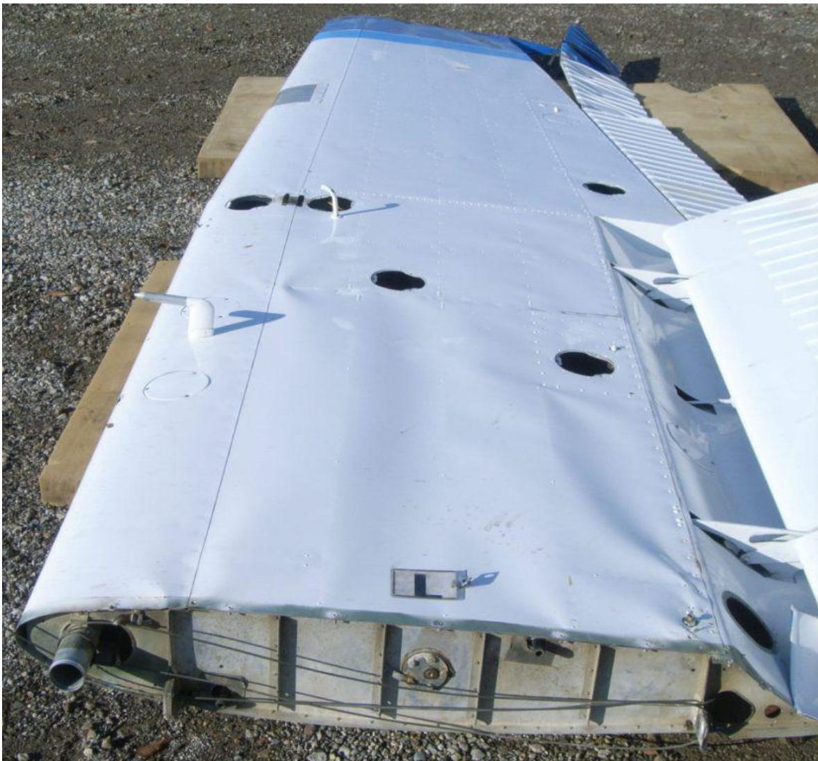
Figure 5 - Left Wing Underside
