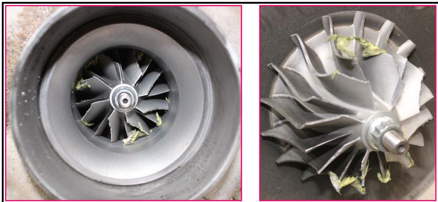
Figure 6: Compressor Wheel (with broken blades and towels residue)
