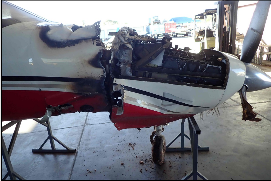
Photo 2 – Smoke Streaks Aft of Firewall
