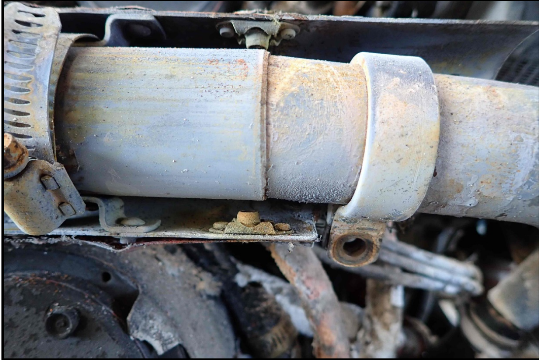
Photo 9 - Intermediate and Right Exhaust Crossover Pipe Engagement
