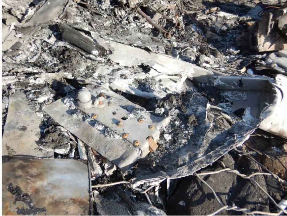
Baggage door latch, NTSB photo
