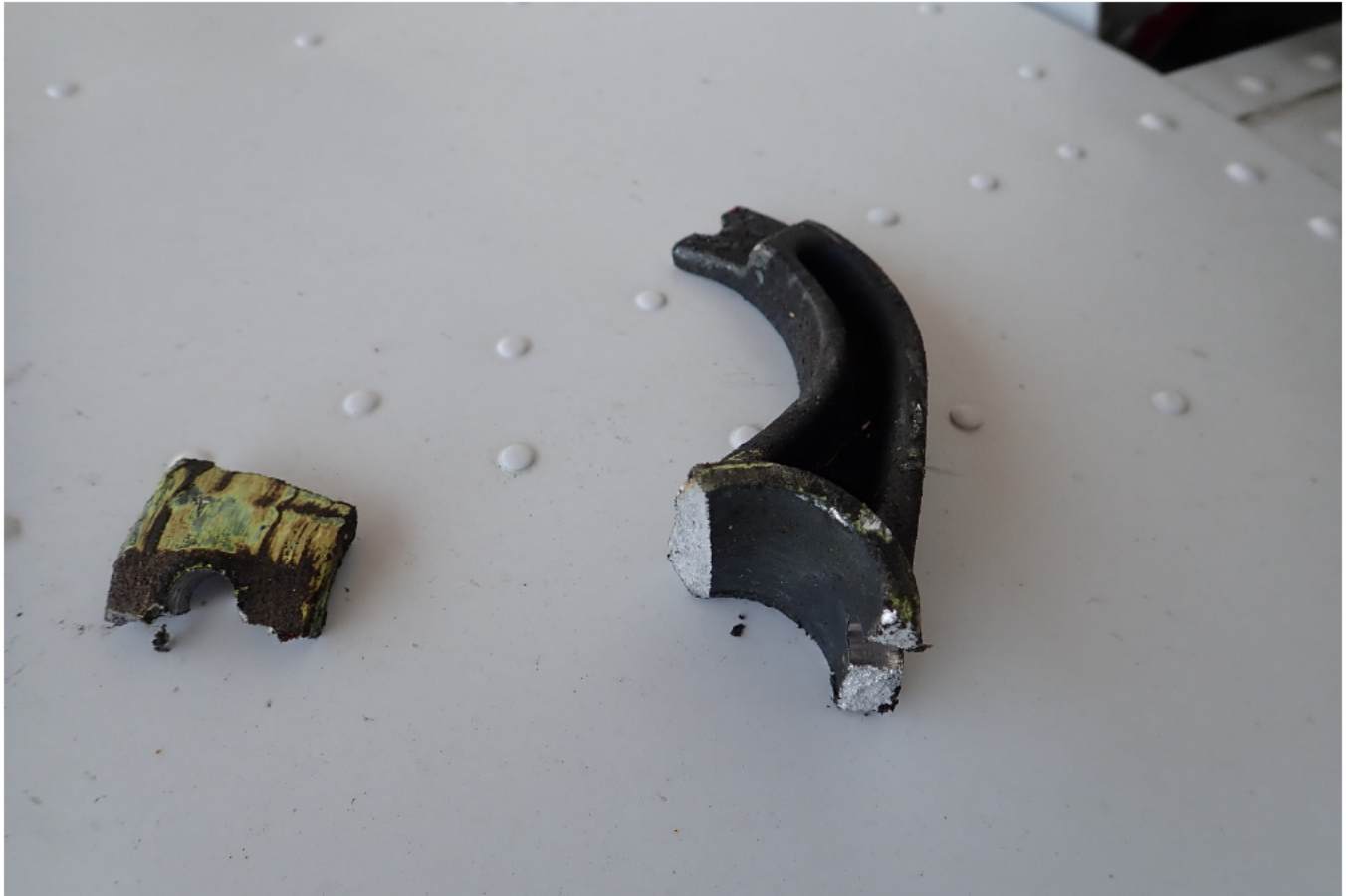
Rudder bellcrank, ASI-19-CI-030
