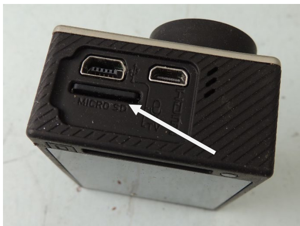
Figure 2. The micro SD card seated properly in the device. The arrow denotes the location of the card.
