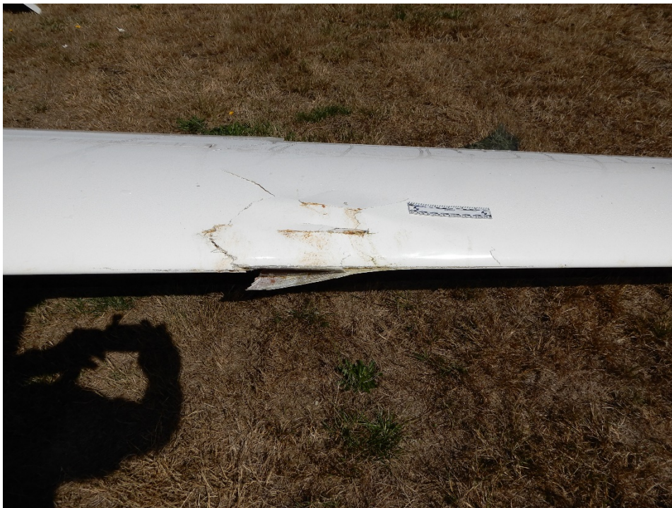
Photo 4. Left wing showing cracks in composite material along with brown colored deposit and pine needles trapped in cracks.
