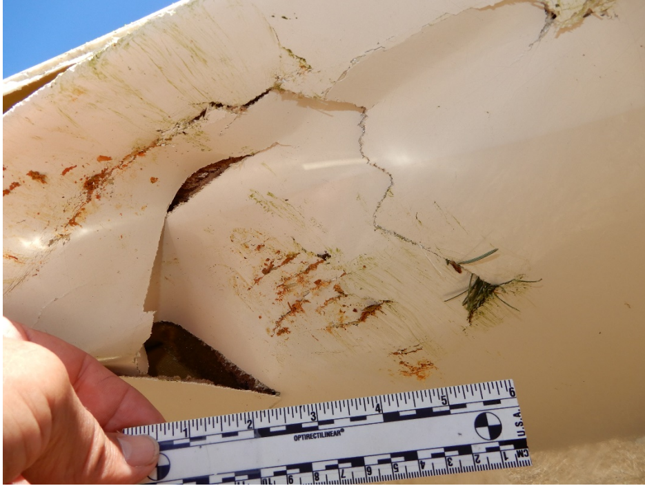
Photo 5. Underside of left wing, showing cracks in composite material, brown colored deposit and pine needles trapped in cracks.
