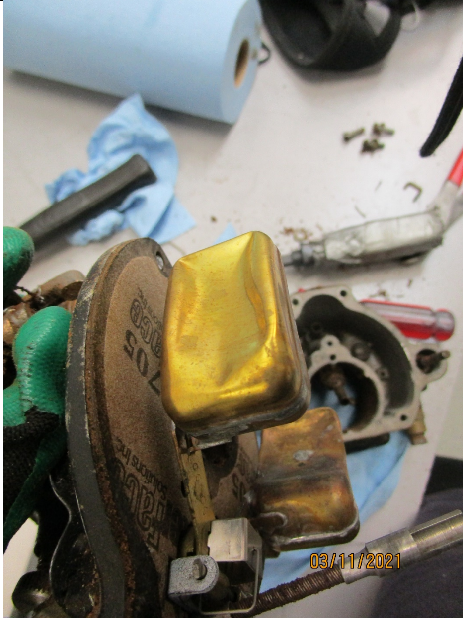
Carburetor was disassembled, both floats appeared to be “crushed”
