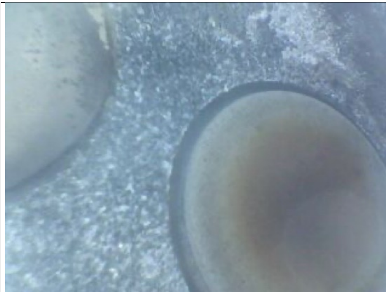
Borescope of the cylinders, showing intake and exhaust valves.
