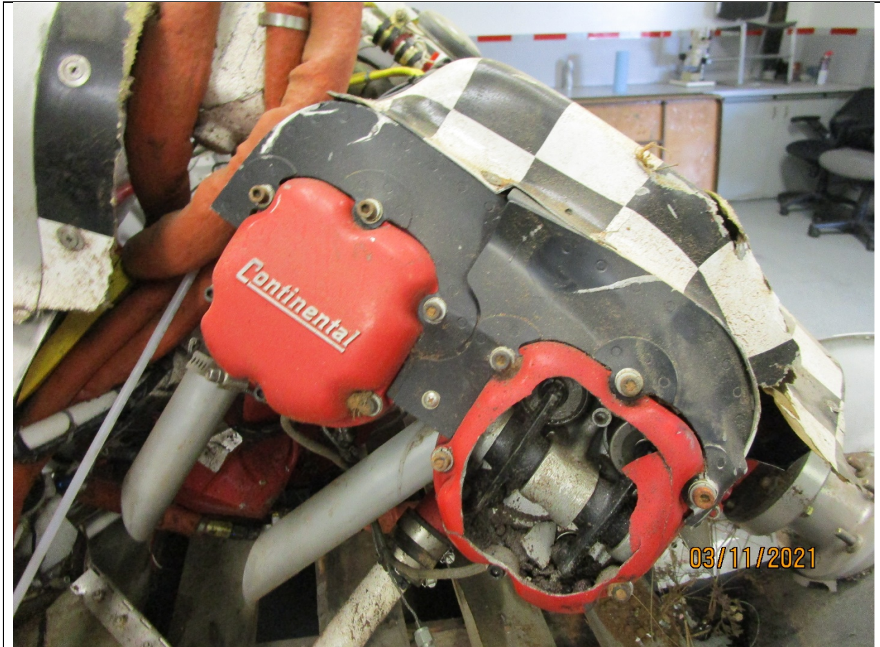
Right side of engine, note damage to the valve cover.
