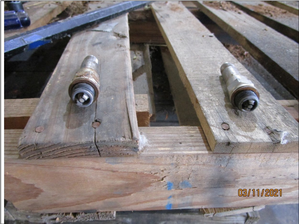
Sparkplugs exhibited normal wear and deposits
