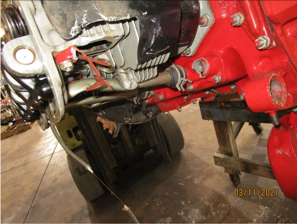
Missing pushrod and tube, the left front cylinder also has a mangled pushrod/tube
