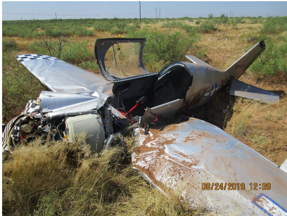
Figure 8: Forward left side of Main Wreckage
