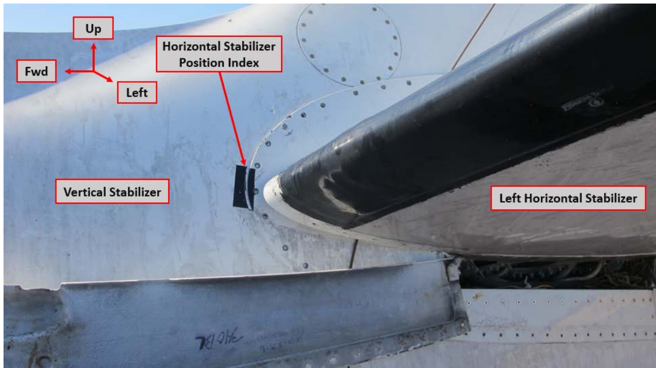
Figure 16 - Horizontal stabilizer position marking in take-off/landing setting
